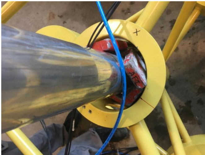
FIGURE 9: Additional weights (red) placed around the foot of tower (photo by Sebastien Gueydon)
