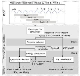
Fig. 2. Illustration of the proposed sea state estimation method, in two main steps. Firstly the point-wise wave spectrum candidates  $\hat{S}_{ij}(\omega, k)$  are computed by solving (5) through iteration. Secondly, the relative wave direction and the spectrum estimates are found by considering the energy in the candidates.
