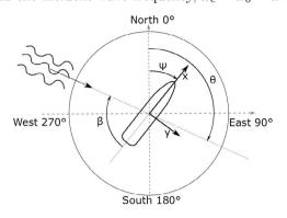
Fig. 1. Definition of the wave propagation direction  $\Theta \in [0, 360)^{\circ}$ , heading of the vessel  $\psi$ , and relative wave direction  $\beta$ . Starboard incident waves have  $\beta \in (-180, 0]^{\circ}$ , and port incident waves have  $\beta \in [0, 180]^{\circ}$ .
