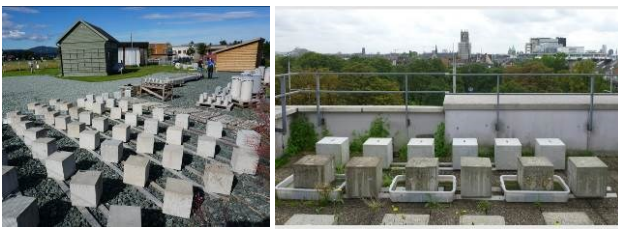
Fig. 7. SINTEF (left - Trondheim, Norway) and VDZ (right – Düsseldorf, Germany) outdoor exposure sites. Cubes are from various projects (PARTNER, COIN Part II, or RILEM TC258-AAA) (photos by Fournier 2016, Borchers 2016).
