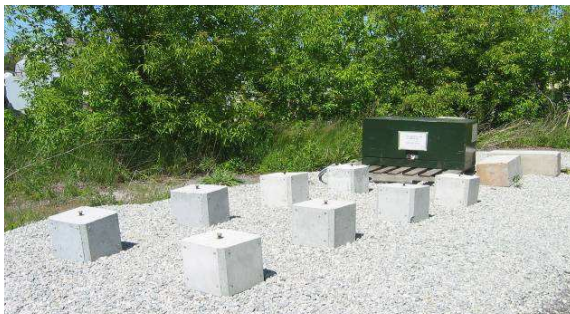
Fig. 15. Concrete specimens on the Leaside outdoor exposure site (courtesy of R.D. Hooton).
