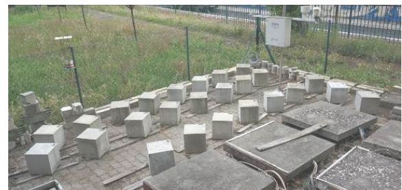
Fig. 6. COIN cubes on the LNEC exposure site in Lisbon (Portugal) (picture by Fournier, 2015).
