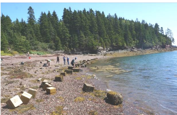
Fig. 8. ASR blocks at low-tide level on the Treat Island cold water marine exposure site. Most recent RILEM TC258-AAA cubes (5) are in the left inside, while CANMET ASR blocks are aligned further down (photo by Fournier, 2017).
