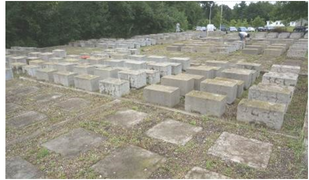
Fig. 16. CANMET exposure site. Blocks and slabs subjected to ASR expansion testing (photo by Fournier, 2015).
