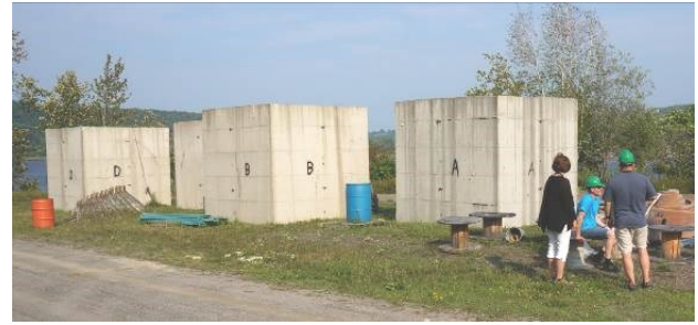
Fig. 19. Monolithic blocks for ASR research at the Mactaquac Generating Station (photo by Fournier, 2017).
