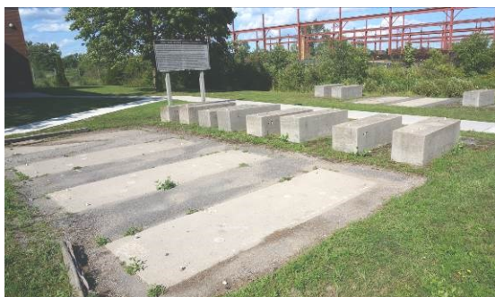
Fig. 12. Concrete specimens incorporating Spratt limestone, Kingston outdoor exposure site (photo by Fournier, 2017).
