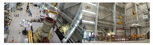
**Figure 1.** The original shrinking fit lift operation to be automated in the project. Screen captures are taken from a video of the assembly [2]. The capture (a) is the view of the operation from above at the time 0:24 and the capture (b) is a side view at the time 0:26 of the video.
