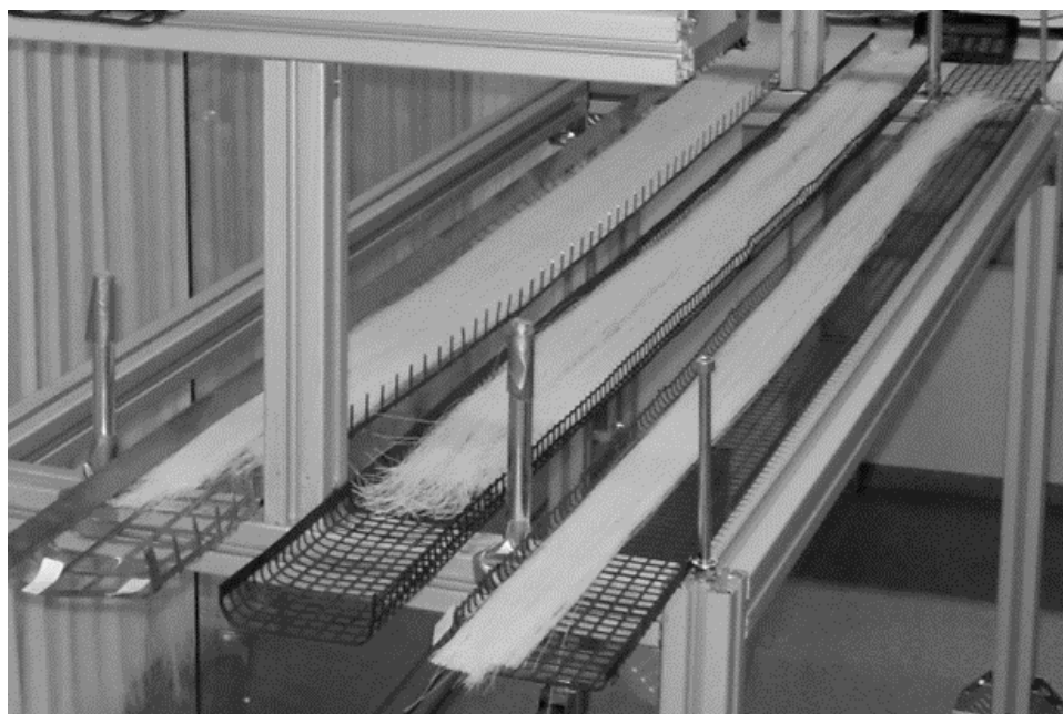
Figure 5. Perforated plates with square openings ( 10 \times 10 \text{ mm}^2 ) and ( 20 \times 20 \text{ mm}^2 ).
