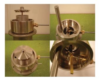
Figure 3.4: Picture of vapor split valve.
