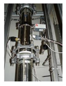
Figure 3.2: Picture of side stream product withdrawal. Swinging funnel leads the liquid from collector outside the column as a product, or back as a reflux.
