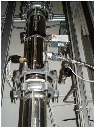
Figure 3.2: Picture of side stream product withdrawal. Swinging funnel leads the liquid from collector outside the column as a product, or back as a reflux.
