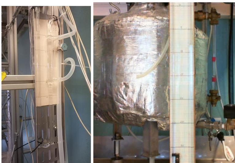
Figure 3.7: Picture of pressure measurements, reboiler and sidestream 2, which works as liquid seals too. It ensures that the vapor is not leaking through the tubes.
