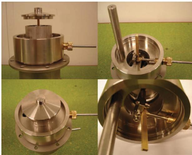
Figure 3.4: Picture of vapor split valve.
