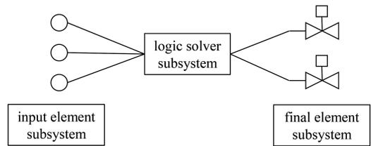
Figure 6. Main parts of a technological barrier.
