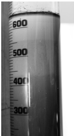
Figure 15 - Zones transformation for lim-wc0.7wp0.5PCE0.18 at 2 h sedimentation after mixing.
