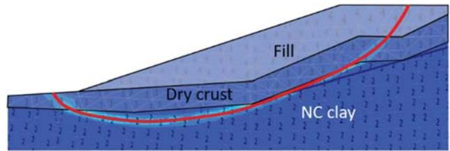
Figure 8. The Vestfossen slope were a fill added in the slope caused failure in the NC clay. Here modelled by using ADPX.
