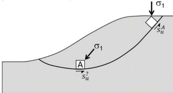
Figure 3. In soli element A the major principal stress is inclined and the shear strength may be closer to  $s_u^A$  than to  $s_u^{DSS}$ .
