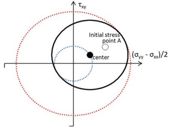
Figure 6. The ADPX yield surface as limited by the maximum and the minimum undrained strength circles around origo. The initial stress is point x. Here:  $B = 3$  and  $\xi/\eta = 1$ .
