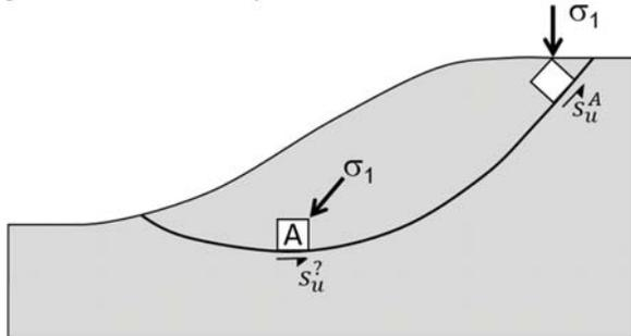
Figure 3. In soli element A the major principal stress is inclined and the shear strength may be closer to  $s_u^A$  than to  $s_u^{DSS}$ .
