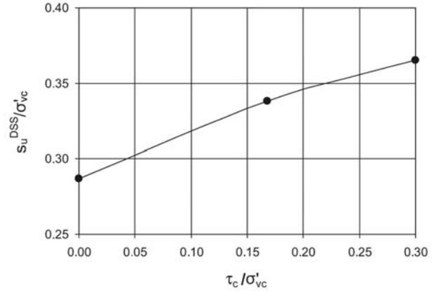
Figure 4. The DSS undrained shear strength increase when consolidated for an inclined, initial effective stress in the direction of undrained loading, Andersen (2009).
