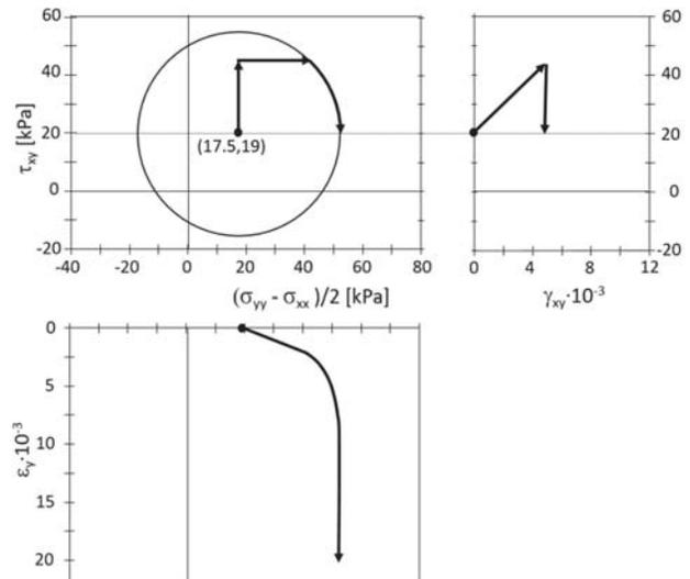
Figure 7. The stress path and stress strain paths obtained from applying shear followed by normal compression.
