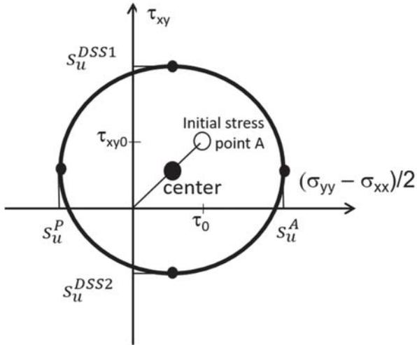
Figure 5. The ADPX yield surface is translated towards point A representing the initial deviatoric stresses. Here:  $\xi = \eta = 0.5$ .
