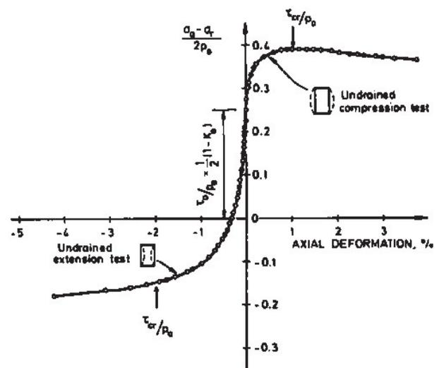
Figure 1. Anisotropic undrained strength Drammen clay (Eide and Bjerrum, 1973).
