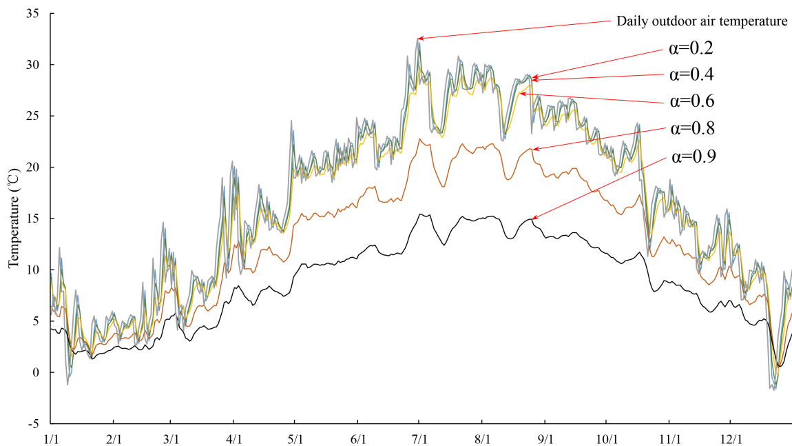
519 520 Figure 9: Effect of different \alpha -values on the equation with a seven-day running mean outdoor external temperature, as 521 proposed by GB/T 50785, for the climate of Shanghai, China.
