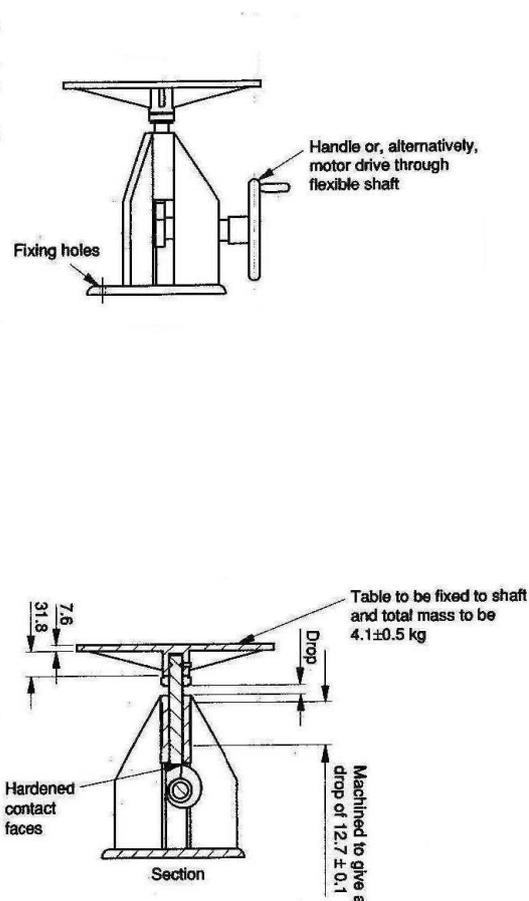
Figure 2: Principal drawing - Flow Table dimensions as described in BS 4551, Part 1, 1998
