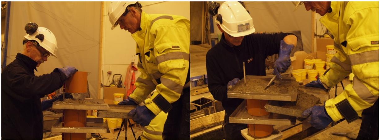
*Figure 3: Sampling from the Settlement Pipe Apparatus*
