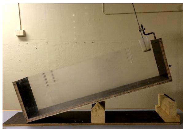
**Evaluation:** The ASTM standard describes that "the test method provides users with a laboratory procedure to determine the potential dynamic segregation of self-consolidating concrete". It implies that it is not designed for building site measurements. However, the principle seems promising and simplifications to meet in-situ measurement requirements should be considered.
