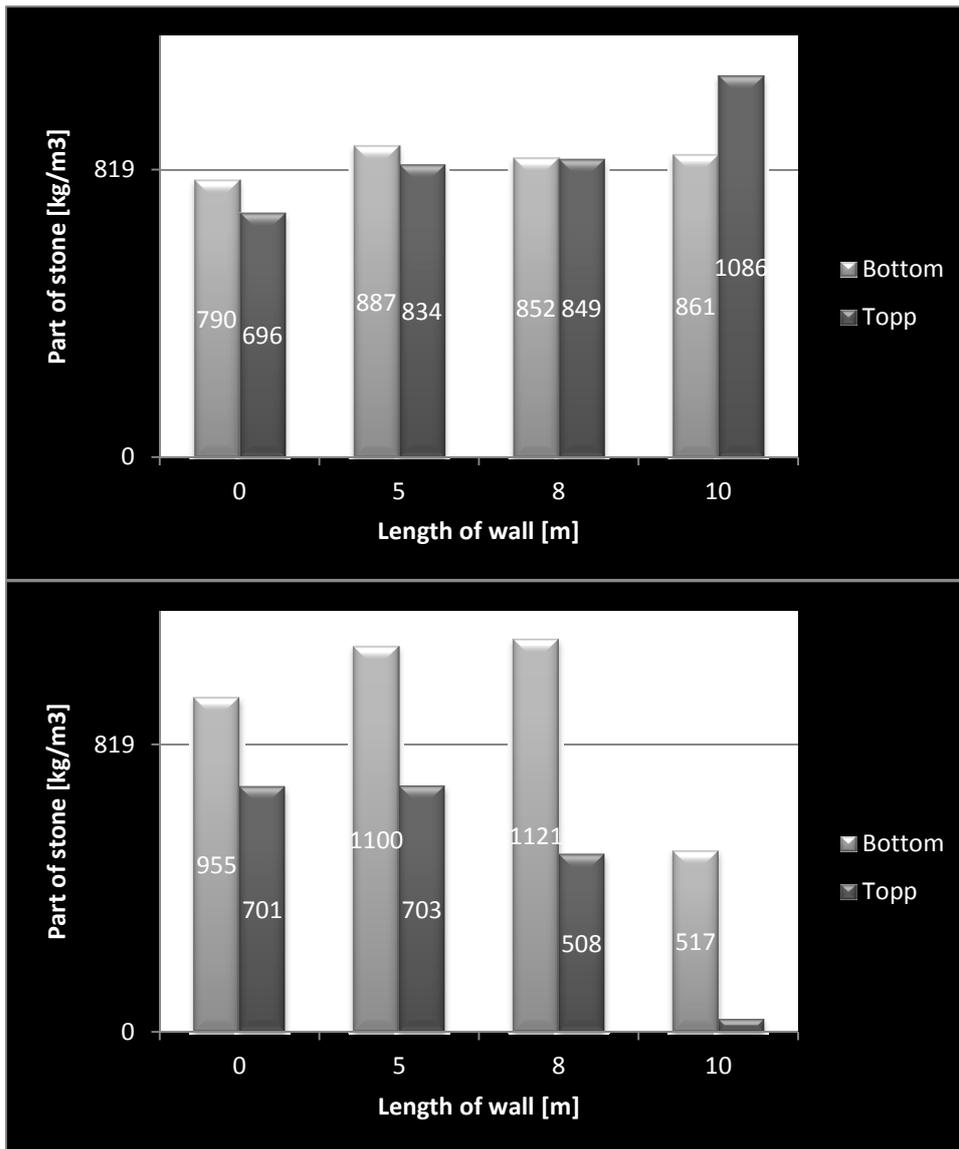
Figure 4 Coarse aggregate content in the selected locations. The coarse aggregate content taken from the mix design is 819 kg/m<sup>3</sup>
