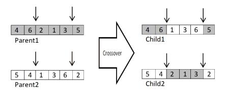
Figure 1. Crossover operation for  $(6 \times 6)$  test problem
