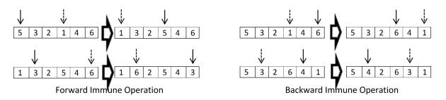
Figure 4. Immune operation for a chromosome of  $(6 \times 6)$  test problem
