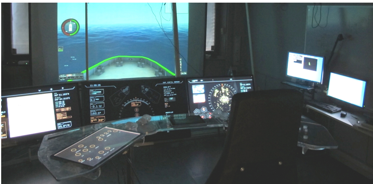
Figure 3 - The design lab in Oslo connected to a ship simulator, source: Ulstein Bridge Concept
