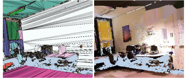
Fig. 11. Textured reconstruction from a Kinect point cloud. The quality of the reconstructed geometry is acceptable, the quality of the textures is poor due to the relatively sparse point density.
