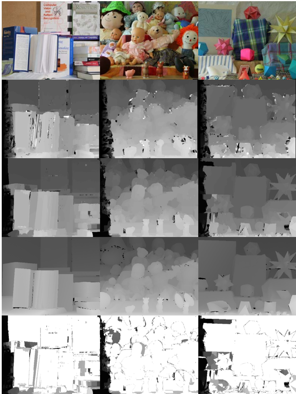
Figure 9: The Comparison of Final Depth Results for the Books, Dolls, and Moebius Stereo Image Pairs (from left to right). Rows from top to bottom: the input left images, results of NCC, final depth results by proposed method, ground truth and “bad pixel” matching results.
