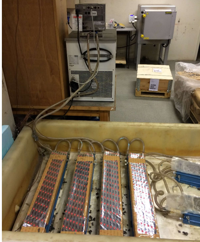
Figure 1. Temperature-controlled moulds connected to a Julabo temperature-control unit: after sealing of the prisms, but prior to placing the insulation and top-cover on the container.
