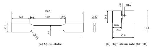
Figure 3.: Specimens geometry for different strain rates.
