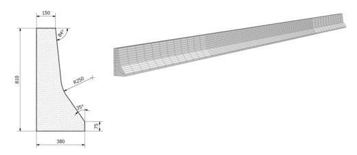
Figure 15.: New Jersey concrete barrier FEM and cross section details.
