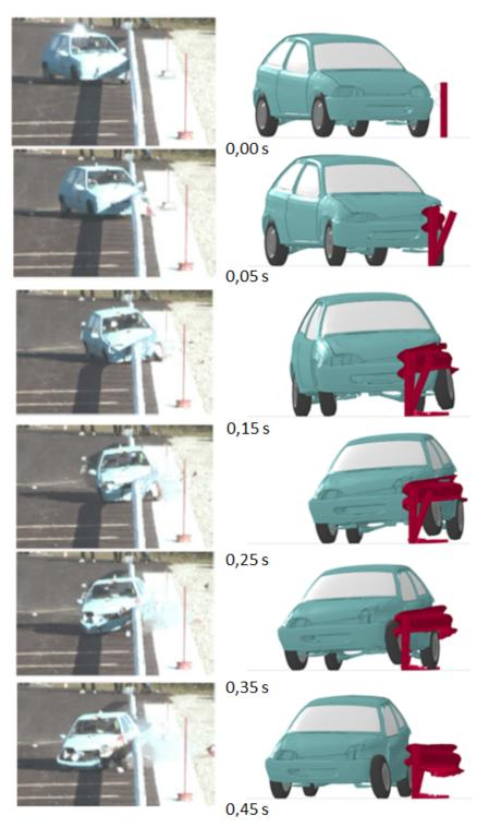
Figure 11.: Comparison between experimental tests, from  $\left[18\right]$  and numerical simulation.
