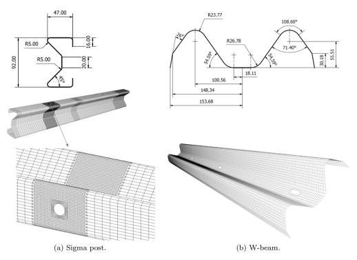
Figure 7.: Finite element mesh for post and beam. Connection area is detailed.
