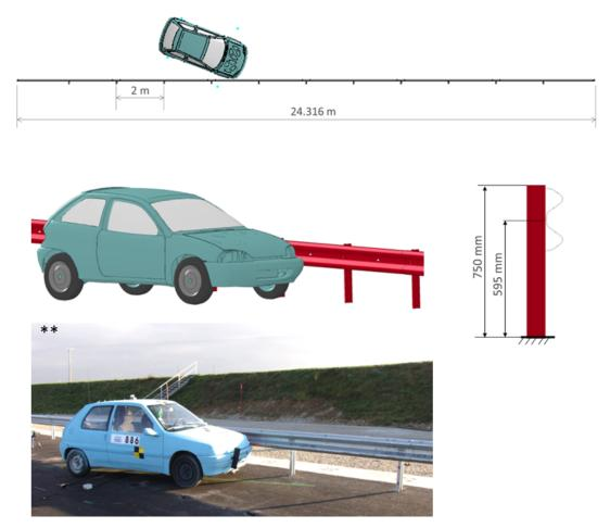
Figure 6.: Vehicle initial condition before impact (extracted from [18]).
