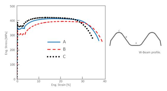
Figure 4.: Quasi-static stress-strain curves for W-beam material.
