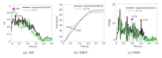
Figure 10.: Severity index history during the car impact with the steel guardrail system.
