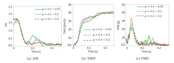
Figure 17.: Severity index history within the car impact with New Jersey concrete barrier system.
