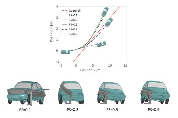
Figure 9.: Impact simulation for different plastic strain limits. Pictures extracted at time instant of 0.273s.
