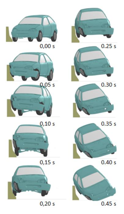
Figure 16.: Simulation of vehicle impact against New Jersey concrete barrier.
