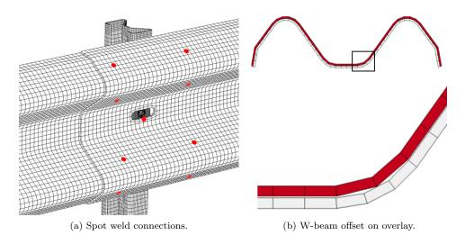
Figure 8.: Post and W-beam connection.
