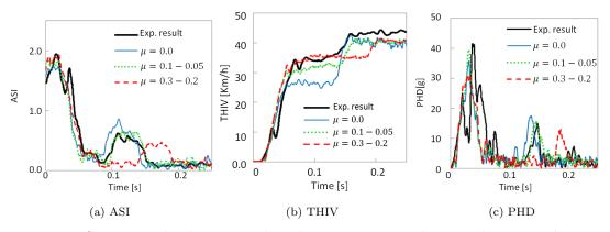
Figure 13.: Severity index history within the car impact with vertical concrete barrier system.
