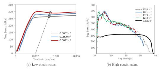
Figure 5.: Stress strain curves at different strain rates.
