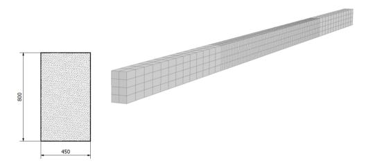
Figure 12.: Concrete barrier geometry and mesh.
