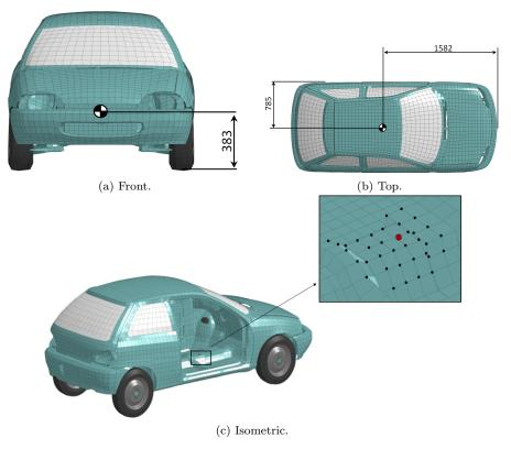
Figure 2.: Car geometry with accelerometer position.
