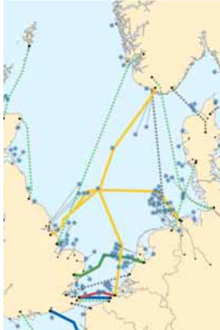
FIGURE 2.2: Proposed topology for MTDC system in the North Sea. Dotted lines are existing HVDC interconnections. Taken from [2]
