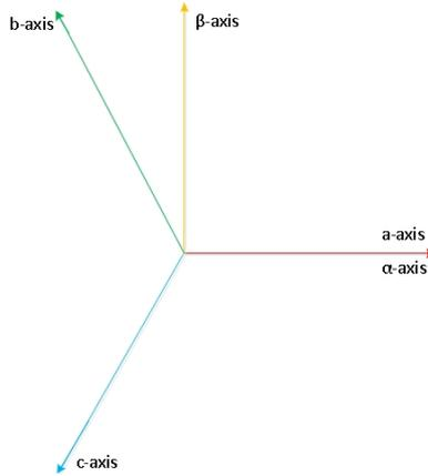
**Figure 5.9:** Three phase and  $\alpha - \beta$  coordinates [44]
