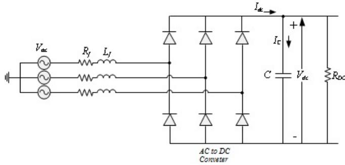
Figure 5.2: Three phase diode bridge rectifier
