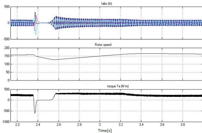
**Figure 9.15:** The impact of three phase to ground fault on the induction motor parameters
