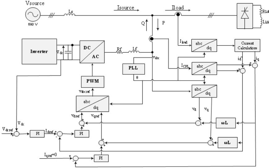
**Figure 5.7:** Control of VSC rectifier [27]
