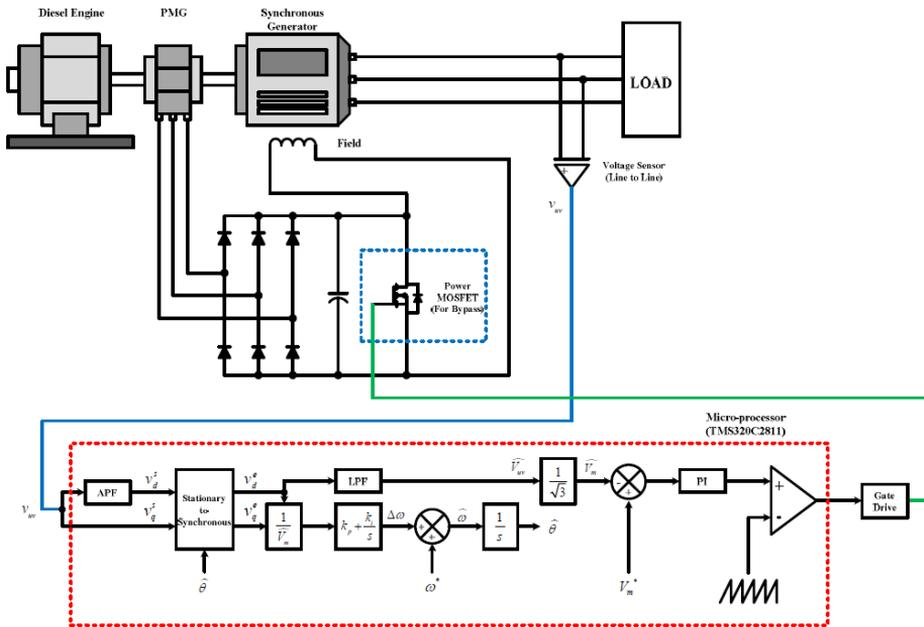
Figure 3.5: Complete block diagram excitation control of ship SG [31]
