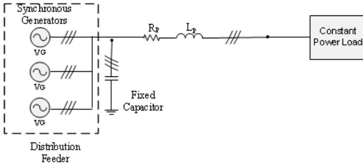
**Figure 6.1:** Parallel operation of three synchronous generators
