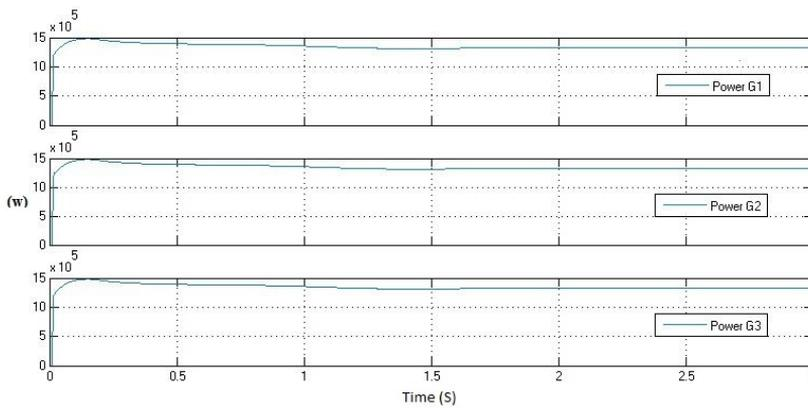
**Figure 6.2:** Power supplied by each generator when operating in parallel
