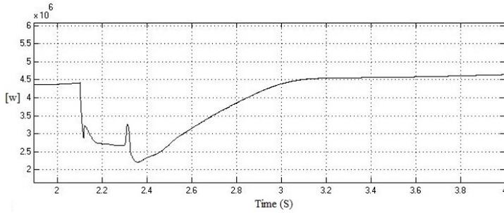
**Figure 9.14:** The power from the system in case of three phase to ground fault
