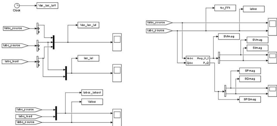
Figure 9.11: The measurements blocks in case of ideal power supply
