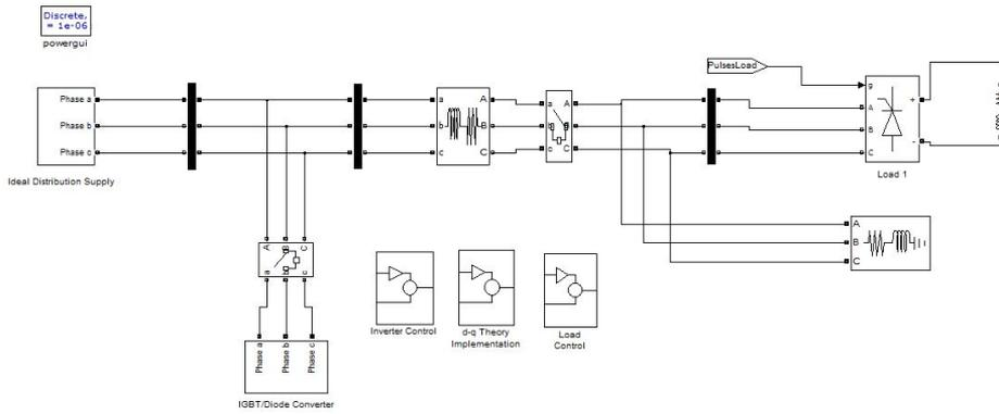
**Figure 9.2:** Simulink model of the system with ideal power supply and non-linear load
