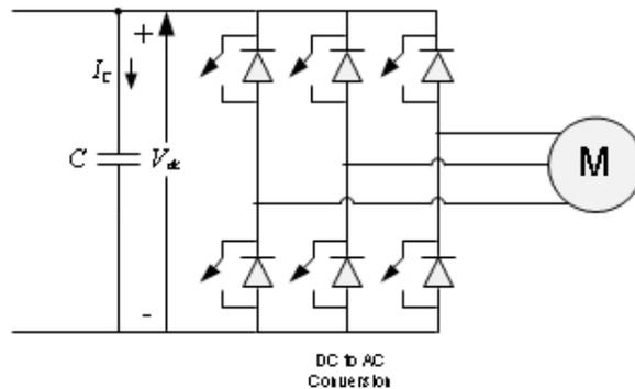
**Figure 3.9:** Circuit diagram of three phase inverter
