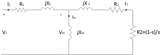
**Figure 3.11:** Induction motor equivalent circuit
