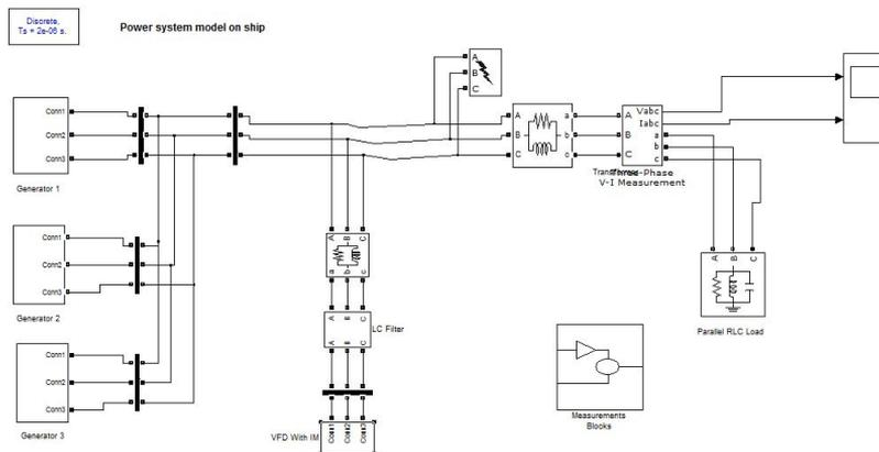
Figure 9.5: Power system on ship with parallel operating generators, one VFD for reactive power control
