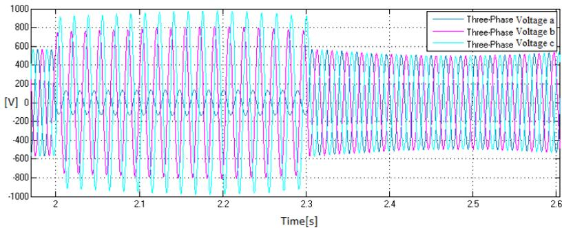
**Figure 2.6:** Voltage swell due to single phase to ground fault with VFD installed in the system
