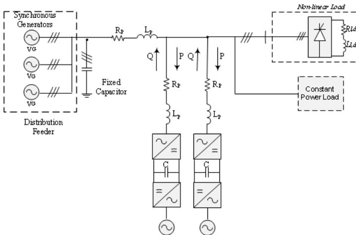
**Figure 6.11:** Power system on ship with two VFDs and non-linear load
