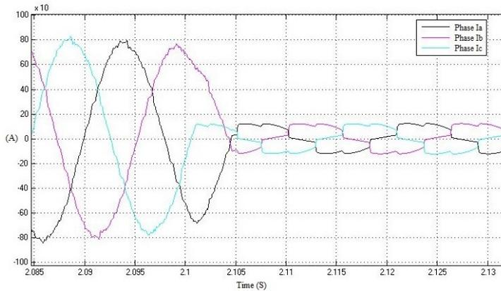
**Figure 6.9:** Three phase source current with and without connecting the VFD
