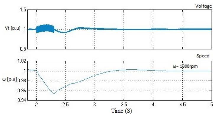
**Figure 9.18:** The impact of three phase to ground fault on SG parameters
