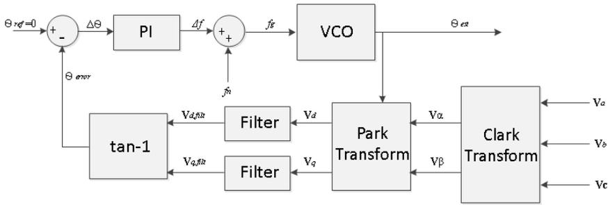
Figure 5.11: Block diagram of Phase Locked Loop [44]
