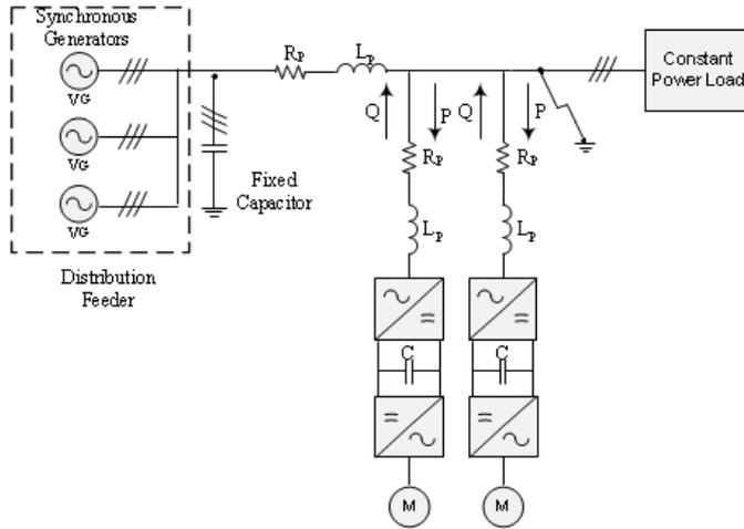
**Figure 6.16:** The power system with two VFDs installed
