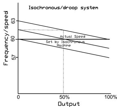
**Figure 3.4:** System with combination of both Isochronous and Droop curves [52]
