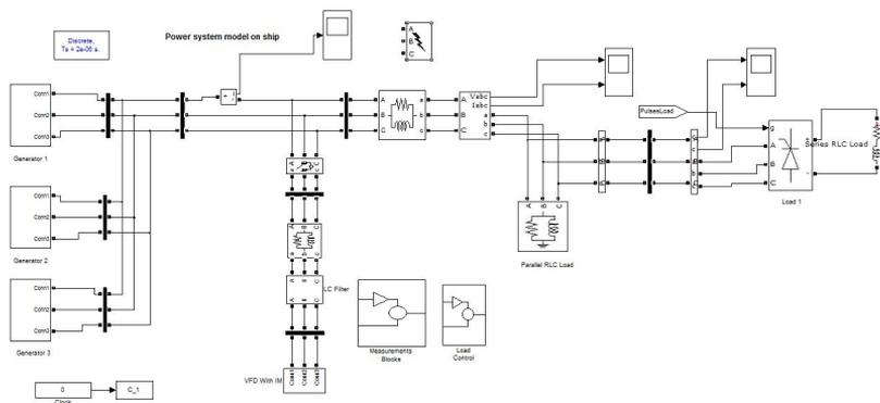
**Figure 9.3:** Power system on ship with parallel operating generators, one VFD and non-linear load
