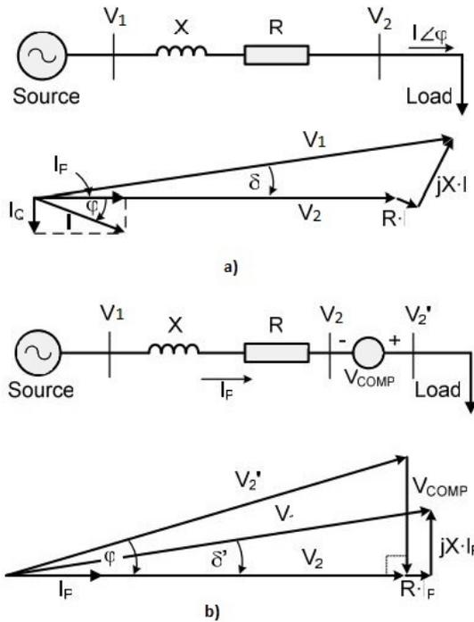
**Figure 9.21:** (a) The system with no compensation (b) The system with series compensation [14]
