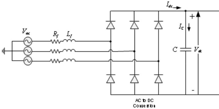
Figure 3.7: Three phase diode rectifier
