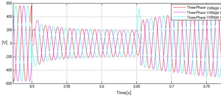
**Figure 4.2:** The voltage dip in case of three phase to ground fault
