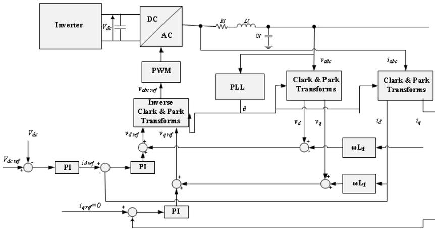
Figure 5.8: Use of Clark and Part transformation in the control of rectifier
