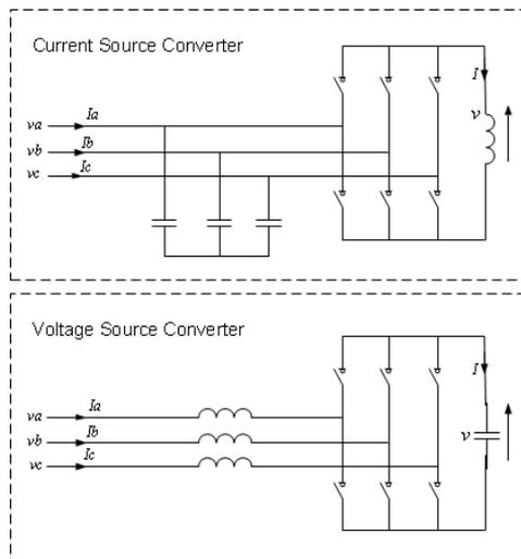
**Figure 9.25:** The VAR compensation with Current souce converter and voltage source converter
