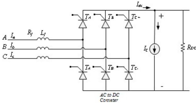
Figure 5.3: Three phase thyristor bridge rectifier
