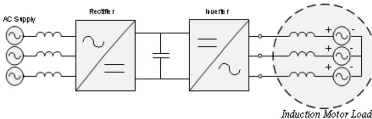
Figure 5.4: Variable frequency drive with IGBT rectifier and inverter
