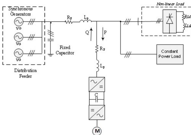
**Figure 6.8:** Power system on ship with one VFD and non-linear load
