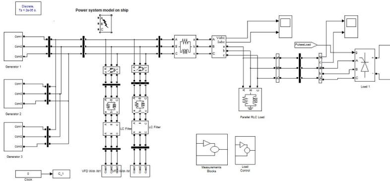
Figure 9.4: Power system on ship with parallel operating generators, two VFDs and non-linear load
