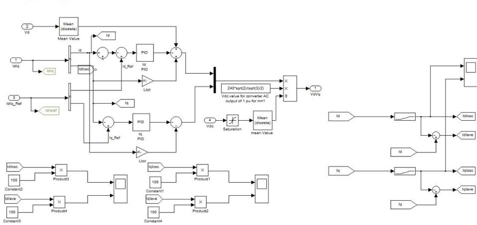
Figure 9.12: The current controller of VSC converter
