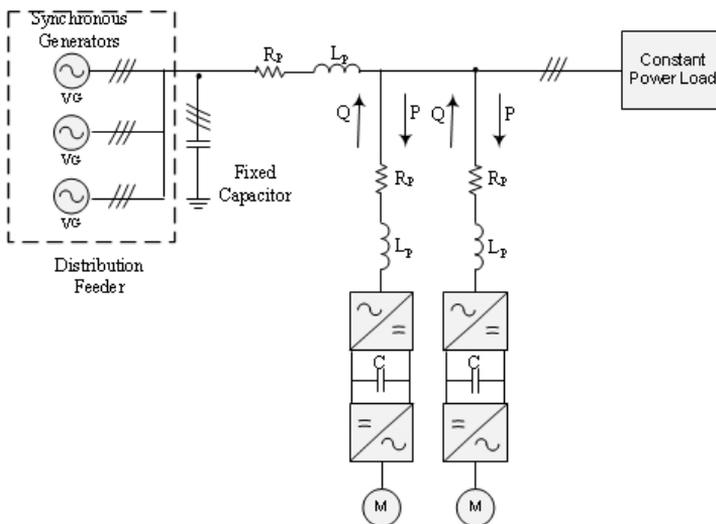
**Figure 3.1:** The general figure of the ship power system comprises of two VFDs
