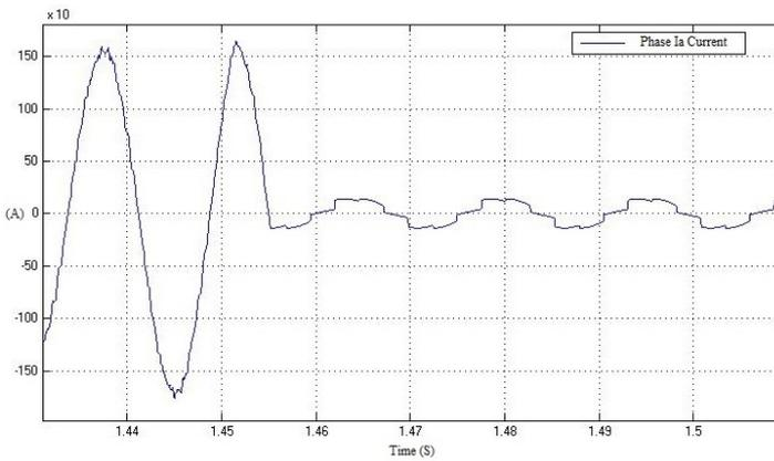
**Figure 6.13:** Single phase source current with and without connecting the VFDs
