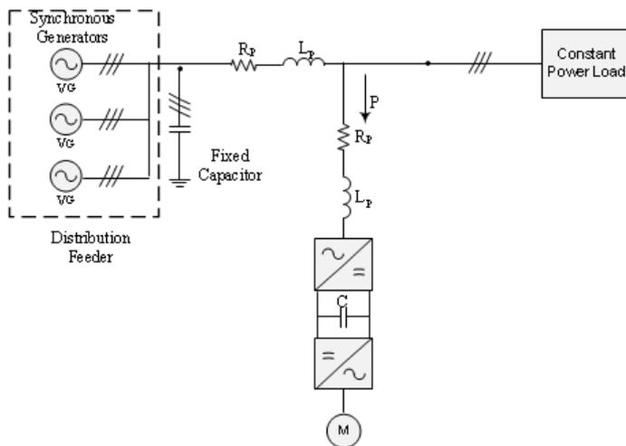
Figure 2.1: General figure of the power system on ship
