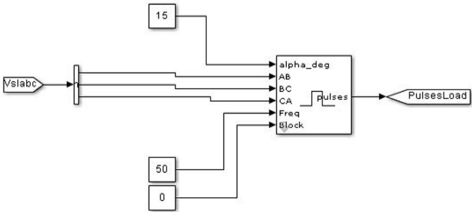
Figure 9.10: The control Block for Thyristor bridge
