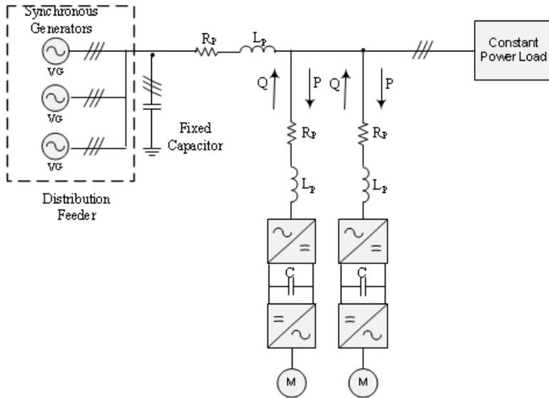
**Figure 1.1:** The typical electric power system topology on the vessel
