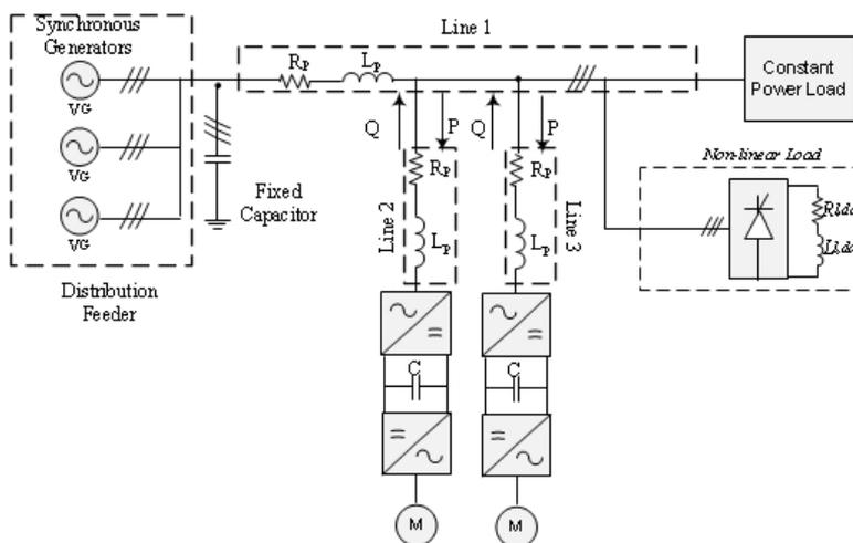
Figure 5.1: General figure of the power system of ship
