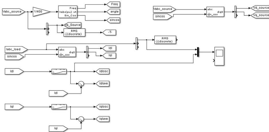
Figure 9.8: Block diagram of implementation of Clark and Park Theory
