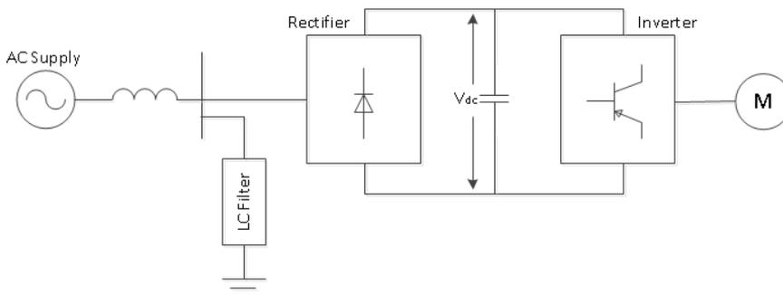
**Figure 2.2:** The general figure of variable frequency drive
