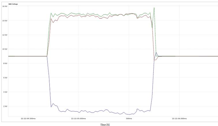
**Figure 4.5:** Voltage swell in case of single phase to ground fault [29]
