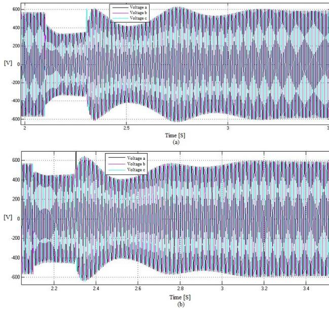
**Figure 6.15:** (a) Three phase to ground fault with no reactive power compensation (b) Three phase to ground fault with reactive power compensation by one VFD
