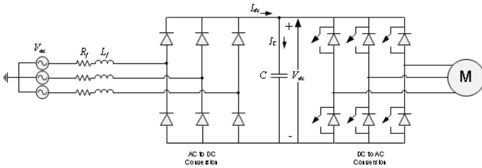
**Figure 3.6:** The variable frequency drive block diagram in general
