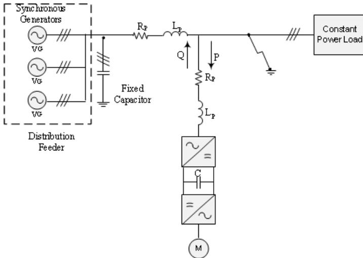
**Figure 6.14:** The power system with one VFD installed
