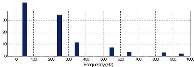
**Figure 4.8:** FFT analysis of current waveform with harmonics
