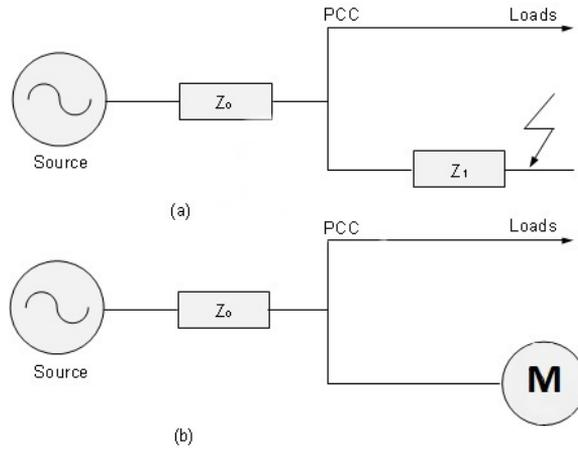
**Figure 4.1:** Representation of fault in power system (a) line fault (b) starting of motor [35]
