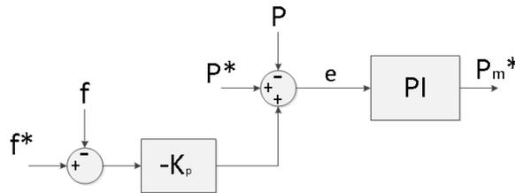
**Figure 5.18:** Frequency droop control with constant power control [18]
