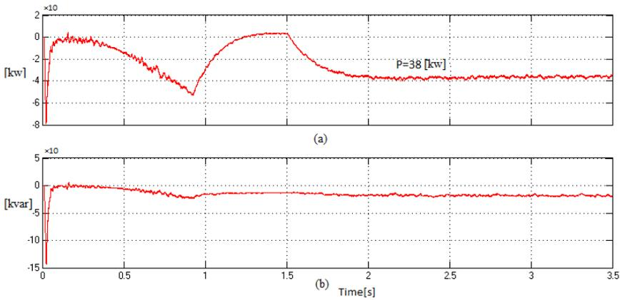
**Figure 2.4:** Impact of induction motor on grid in shape of active and reactive power
