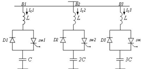
**Figure 9.23:** Thyristor-diode switched capacitor compensation [29]
