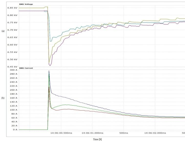
**Figure 4.4:** Starting of induction motor (a) voltage dip (b) starting current [29]
