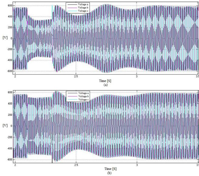
**Figure 6.17:** (a) Three phase to ground fault with no reactive power compensation (b) Three phase to ground fault with reactive power compensation by two VFDs
