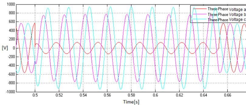
**Figure 2.5:** Voltage swell due to single phase to ground fault without VFD in the system
