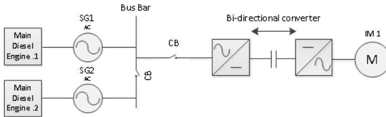
Figure 3.2: Parallel operation of generators in ship electric system
