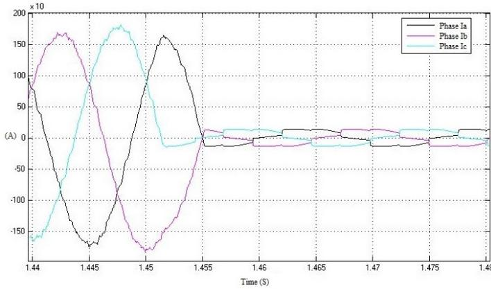
**Figure 6.12:** Three phase source current with and without connecting the VFDs
