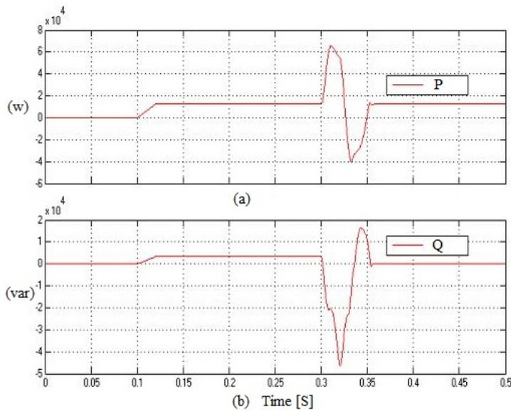
**Figure 9.17:** (a)The real power from the system connected with ideal power supply when converter start compensating the reactive power at  $t= 0.3$  sec (b) Reactive power drawn from the system with ideal power supply when converter start compensating the reactive power at  $t= 0.3$  sec
