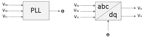
Figure 5.12: Phase Locked Loop block [44]
