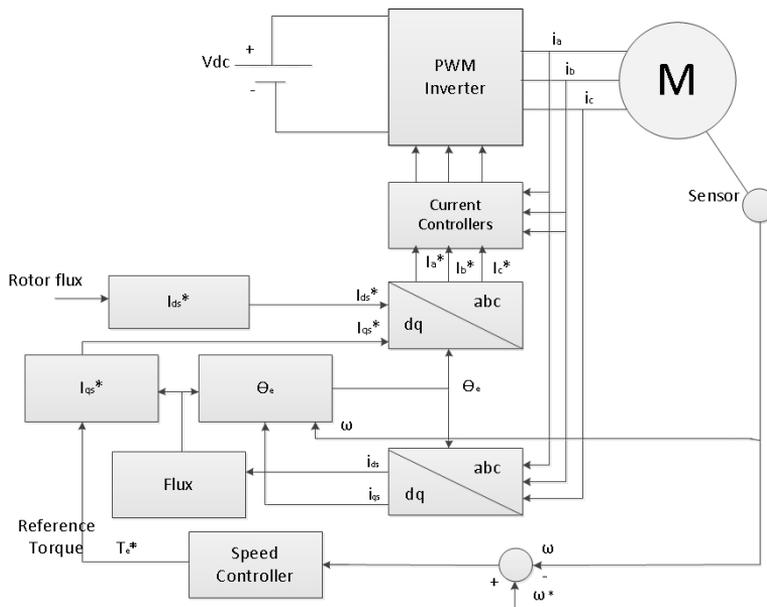
**Figure 5.16:** Control scheme for inverter of variable frequency drive
