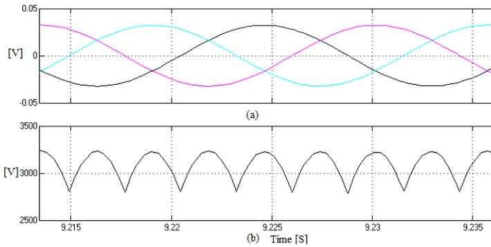
Figure 3.8: Voltage waveform before and after rectification
