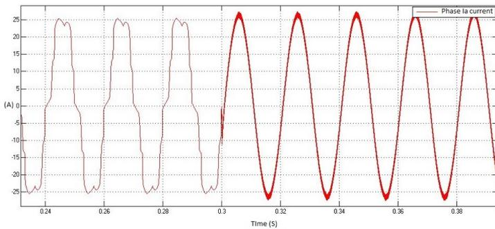
Figure 6.6: Single phase source current before and after harmonics compensation
