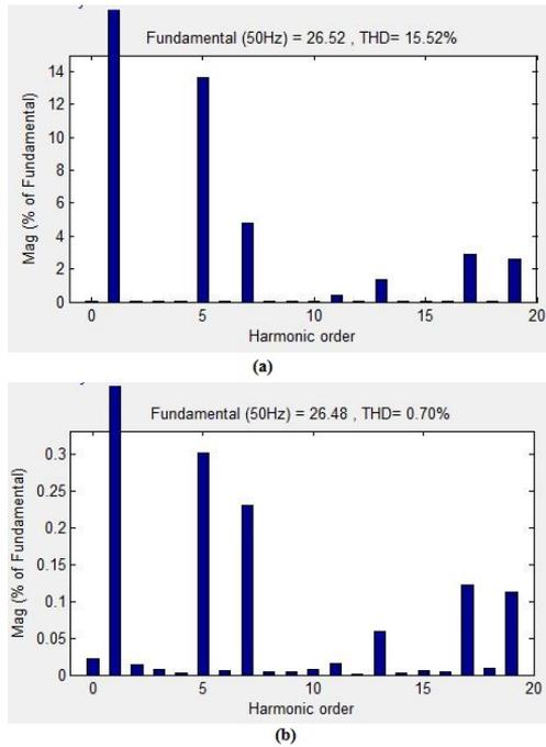
**Figure 6.7:** (a) FFT analysis before connecting the converter (b)FFT analysis after connecting the converter
