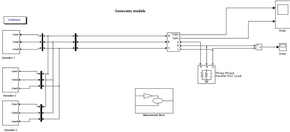
Figure 9.1: Block diagram of parallel operating synchronous generators with parallel RLC load
