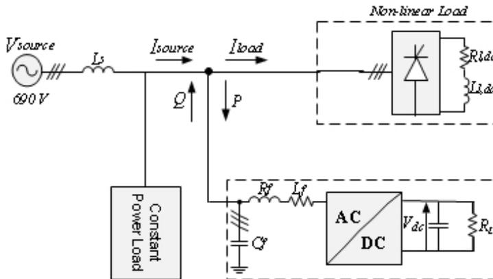
**Figure 6.4:** Power system with ideal supply and non-linear load
