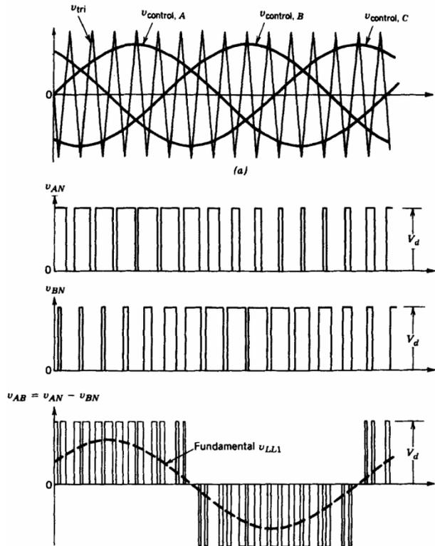
Figure 3.10: Three phase inverter waveform with PWM [49]
