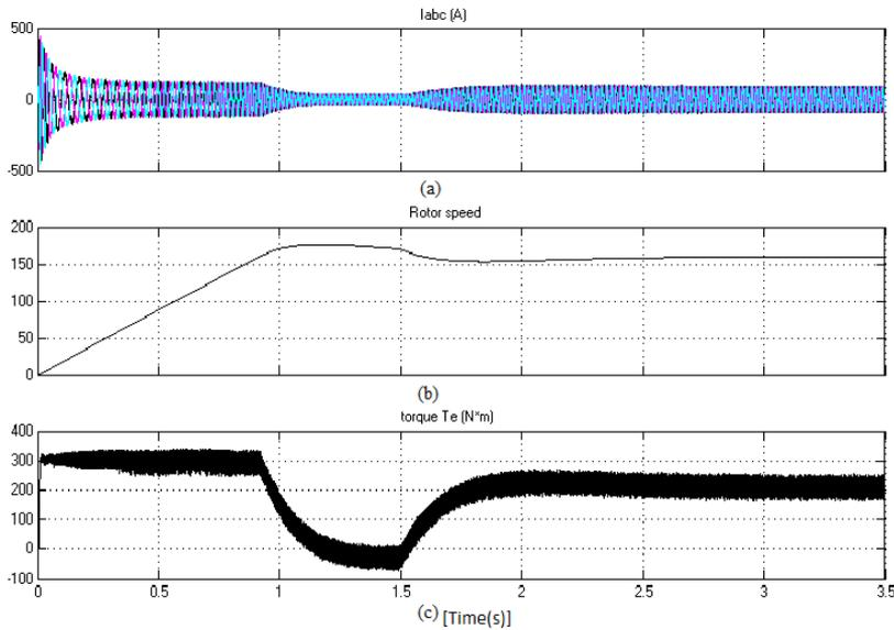
Figure 2.3: Induction motor variables when connected with VFD
