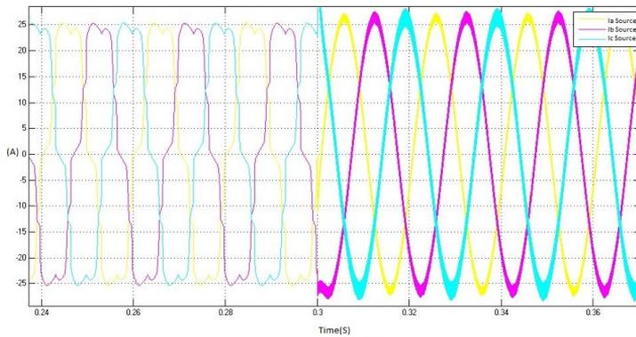
Figure 6.5: Three phase source current before and after connecting the converter
