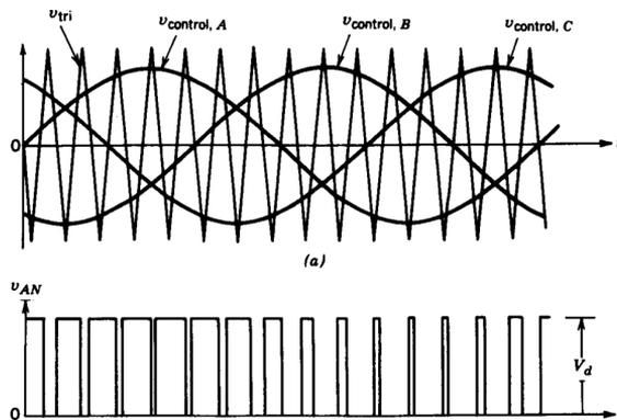
Figure 5.17: Pulse width modulation waveform [49]
