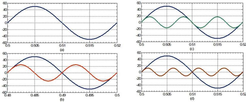
**Figure 4.6:** Comparison of Harmonic and fundamental components of the voltage (a)fundamental component (b) second harmonic with fundamental component (c) third harmonic and fundamental component (d) fourth harmonic and fundamental component
