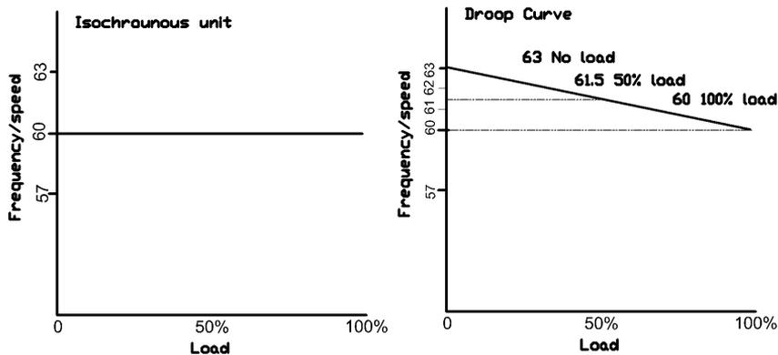
Figure 3.3: Typical figures of Isochronous unit and 5% Droop curve [52]
