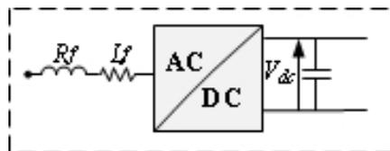
**Figure 5.6:** The block diagram of rectifier used for the modelling
