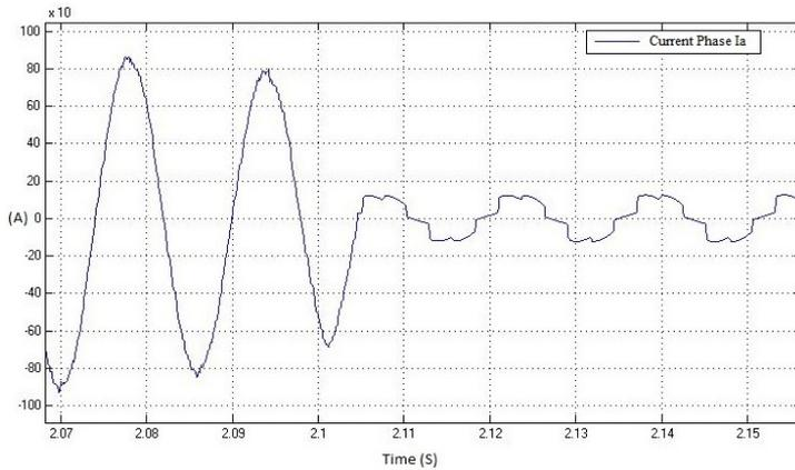
**Figure 6.10:** Single phase source current with and without connecting the VFD
