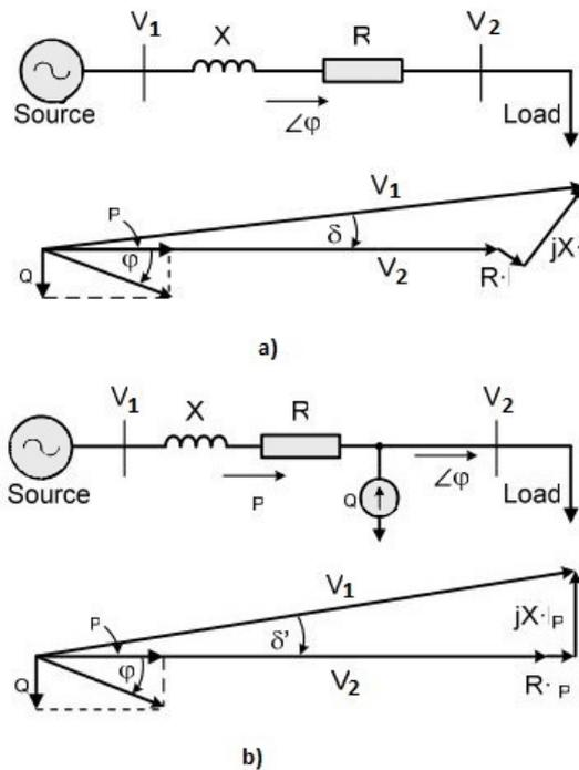
**Figure 9.20:** (a) The system with no compensation (b) The system with shunt compensation [14]
