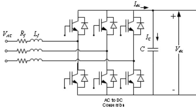
**Figure 5.5:** Circuit diagram of IGBT based rectifier used in the VFD
