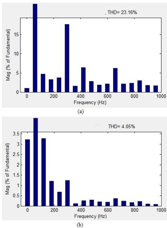
**Figure 9.19:** (a) The FFT analysis without connecting VFD in the system (b)The FFT analysis with one VFD connected in the system
