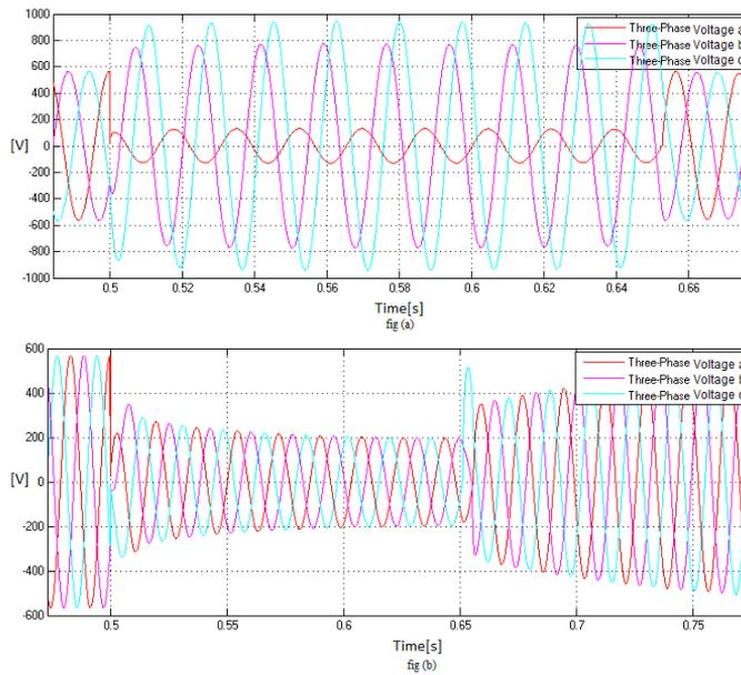
**Figure 4.3:** The voltage dips due to different types of fault (a) The asymmetrical fault due to single phase to ground fault (b) The symmetrical fault due to three phase to ground fault
