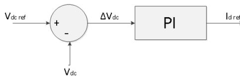
**Figure 5.14:** DC voltage control block
