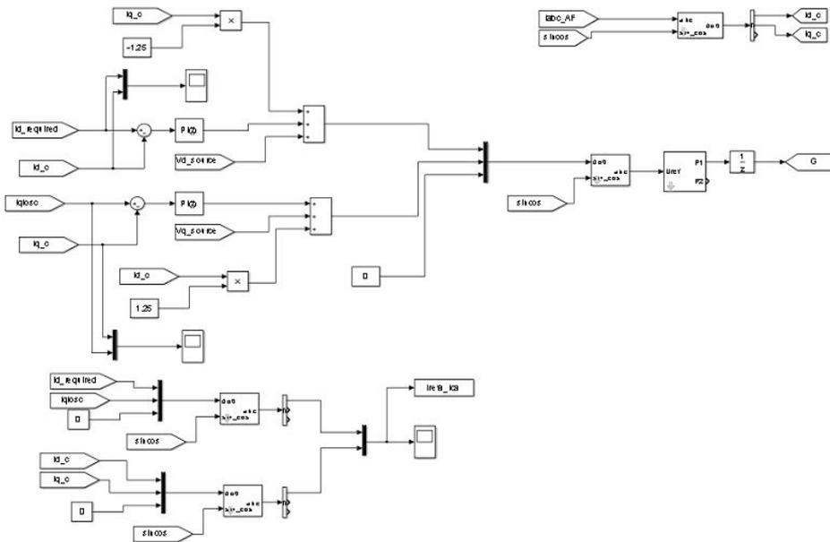
Figure 9.9: The current controller for the harmonics compensation
