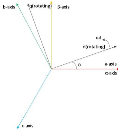
**Figure 5.10:** Three phase coordinate system,  $\alpha - \beta$  coordinates and  $d-q$  coordinated systems. [44]
