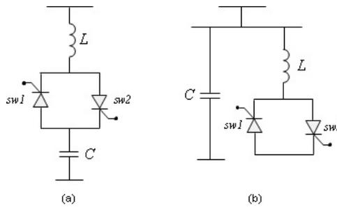
**Figure 9.22:** (a) Thyristor controlled capacitor circuit (b) Thyristor controlled reactor circuit [29]
