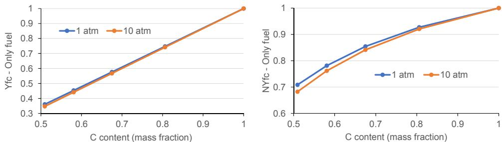
Figure 1: Fixed carbon yield and normalized fixed carbon yield, as a function of carbon content in the biomass, at a temperature of 673 K and at a pressure of 1 and 10 atm.
