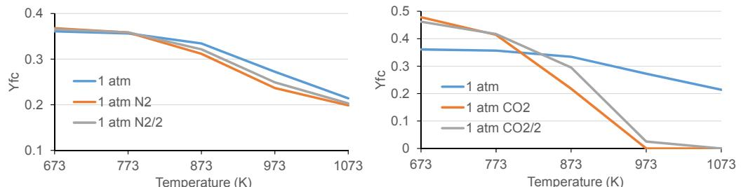
Figure 4: Fixed carbon yield as a function of temperature and carrier gas choice and amount (1 atm: no carrier gas,  $\text{N}_2$  or  $\text{CO}_2$ : carrier gas addition,  $\text{N}_2/2$  and  $\text{CO}_2/2$ : halved molar addition of  $\text{N}_2$  or  $\text{CO}_2$ ) at a pressure of 1 atm.
