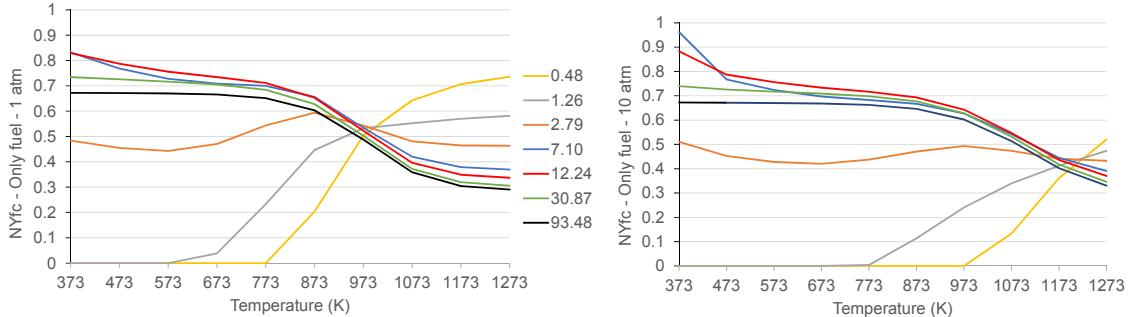
Figure 2: Normalised fixed carbon yield as a function of temperature and O/H ratio (0.48-93.48) for a constant carbon content in the feedstock, at a pressure of 1 and 10 atm.
