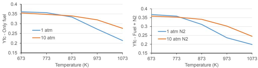
Figure 5: Fixed carbon yield as a function of temperature and pressure, with and without inert carrier gas.
