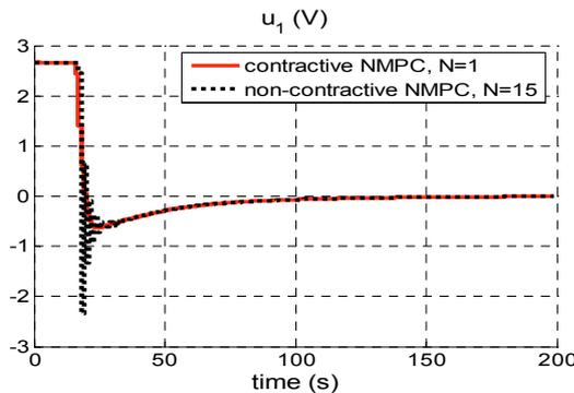
Fig. 2. The control input for subsystem  $S_1$  - case a).
