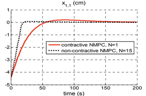
Fig. 8. The state  $x_{1,1} = h_1 - h_1^*$  of subsystem  $S_1$  - case b).
