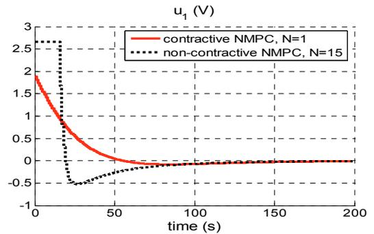
Fig. 6. The control input for subsystem  $S_1$  - case b).
