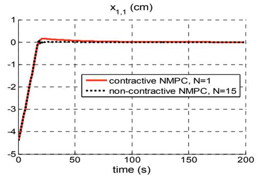
Fig. 4. The state  $x_{1,1} = h_1 - h_1^*$  of subsystem  $S_1$  - case a).
