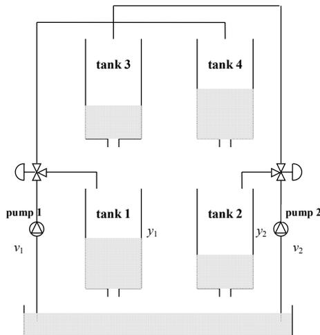
Fig. 1. Quadruple-tank system (Johansson (2000)).
