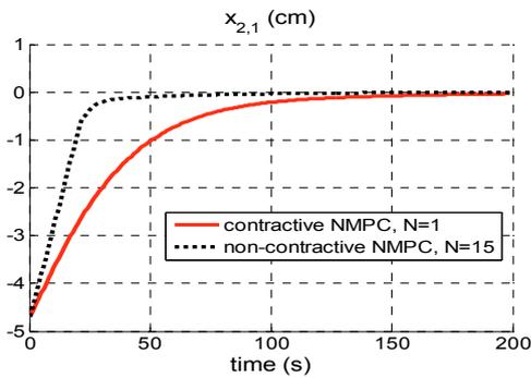
Fig. 9. The state  $x_{2,1} = h_2 - h_2^*$  of subsystem  $S_2$  - case b).
