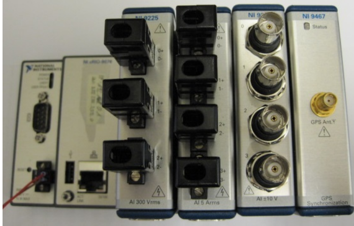
Figure 4.4: The compactRIO, programmed as a PMU, utilized for performing measurements. The chassis is containing the controller, power supply, and Ethernet connection on the left; the voltage, current and low voltage input modules in the middle; and the GPS module at the right.
