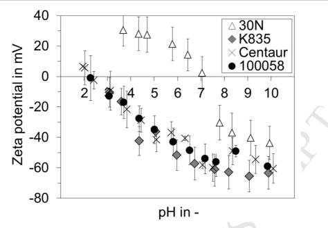
1135Figure 2:Zeta potentials of the fresh 100058, 30N, K835 and Centaur GACs at1136different pH. Error bars represent the standard deviation of three
