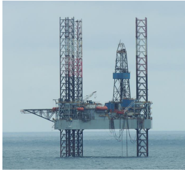
Figure 2.1 - Jack-up rig in the North Sea
