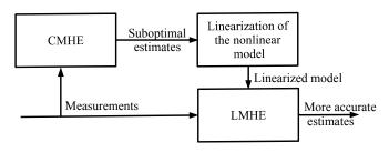
Fig. 1. Schematic overview of the proposed double MHE
