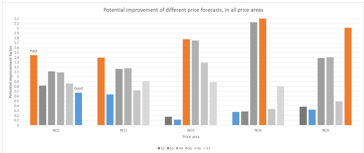
Figure 27 - Price forecast accuracy in different price areas used for price independent bidding. One optimization every second month, starting January 2013, in each price area. Total 30 optimizations. Price scenario 2 - 8.
