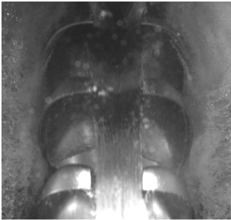
Figure E.45: 70m head, Nozzle open- ing=10mm, n_{11} = 41
