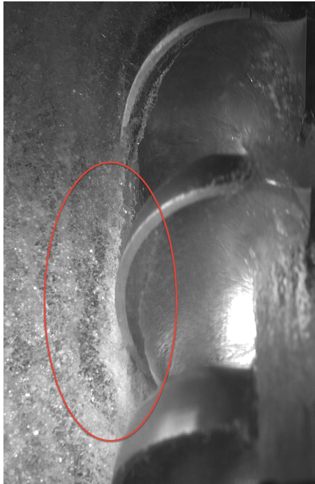
Figure 6.6: First design, 21 buckets, 70m head, Q_{11} = 0.020 , n_{11} = 41
