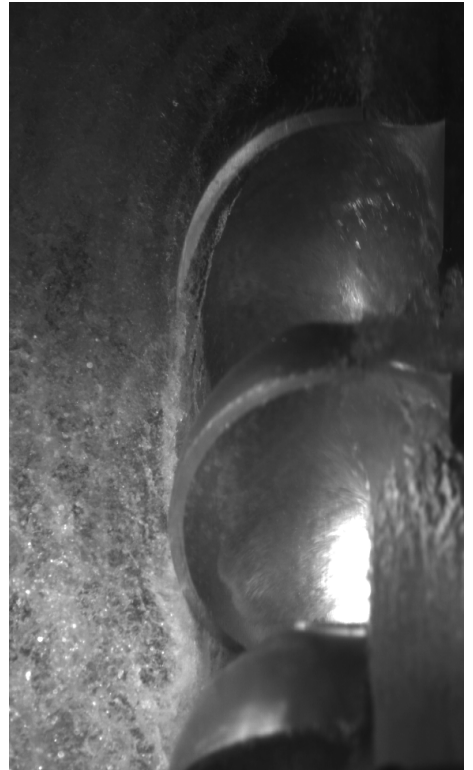
Figure E.4: 70m head, Nozzle opening=18mm, n_{11} = 41
