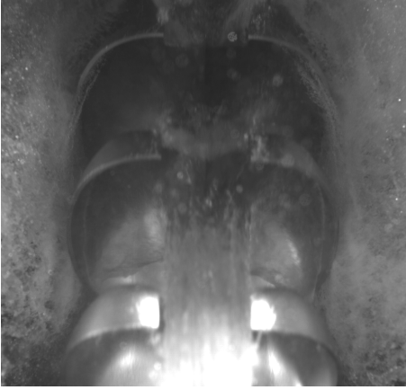
Figure E.39: 70m head, Nozzle opening=12mm, n_{11} = 44
