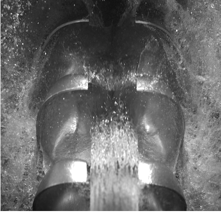
Figure E.19: 25m head, Nozzle open- ing=14mm, n_{11} = 38,5
