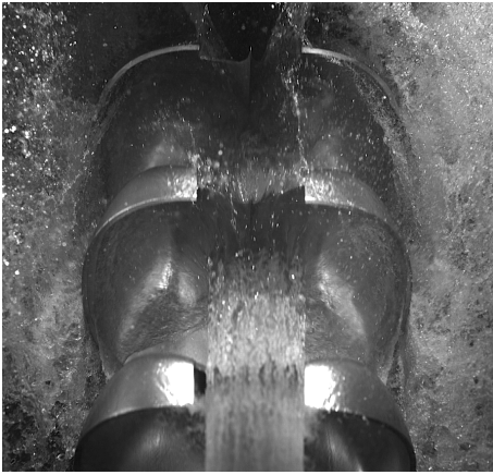
Figure E.17: 25m head, Nozzle open- ing=10mm, n_{11} = 38,5
