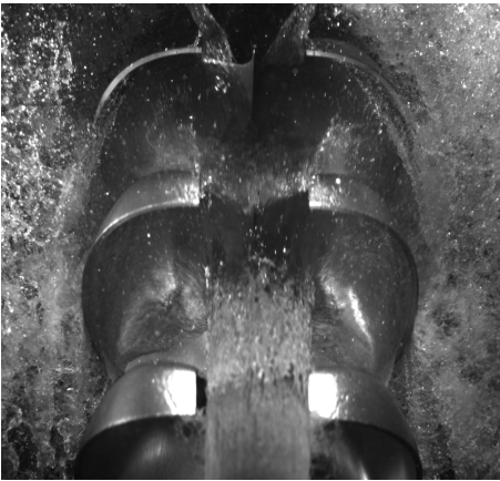
Figure E.25: 25m head, Nozzle open- ing=12mm, n_{11} = 41
