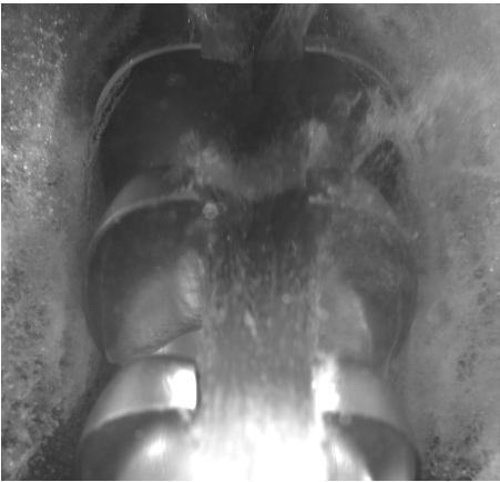
Figure E.41: 70m head, Nozzle opening=16mm, n_{11} = 44
