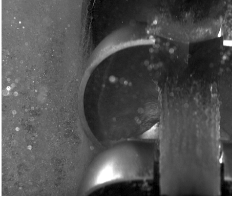
Figure E.9: 70m head, Nozzle opening=14mm, n_{11} = 41
