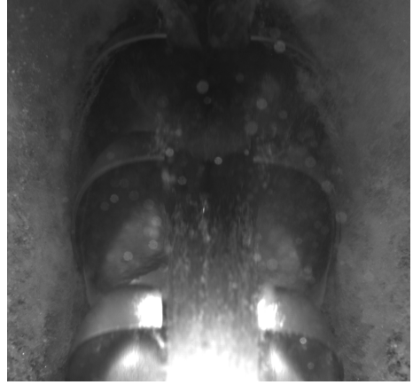
Figure E.48: 70m head, Nozzle opening=16mm, n_{11} = 41
