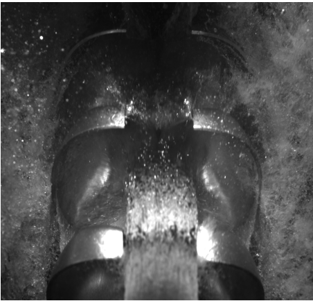
Figure E.21: 25m head, Nozzle open- ing=18mm, n_{11} = 38,5
