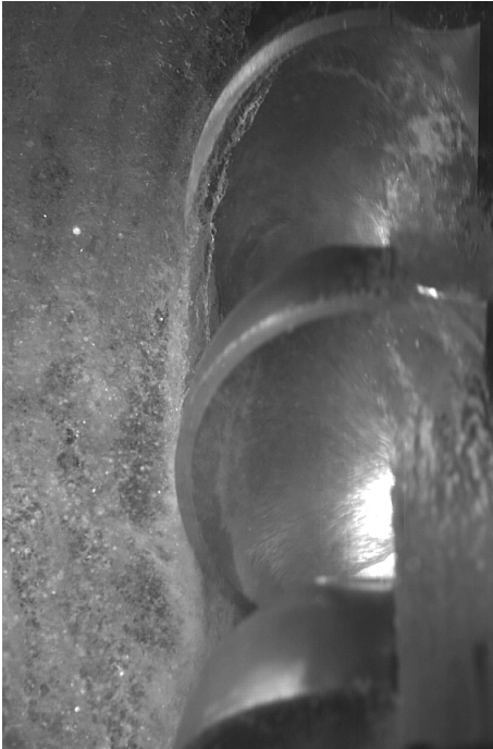
Figure E.5: 70m head, Nozzle open- ing=22mm, n_{11} = 41
