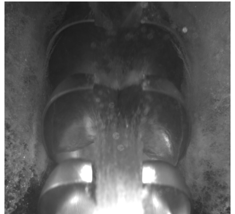
Figure E.38: 70m head, Nozzle opening=10mm, n_{11} = 44
