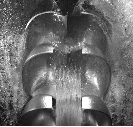
Figure E.23: 25m head, Nozzle open- ing=8mm, n_{11} = 41
