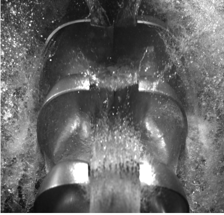
Figure E.27: 25m head, Nozzle open- ing=16mm, n_{11} = 41
