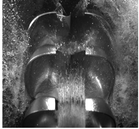
Figure E.24: 25m head, Nozzle open- ing=10mm, n_{11} = 41
