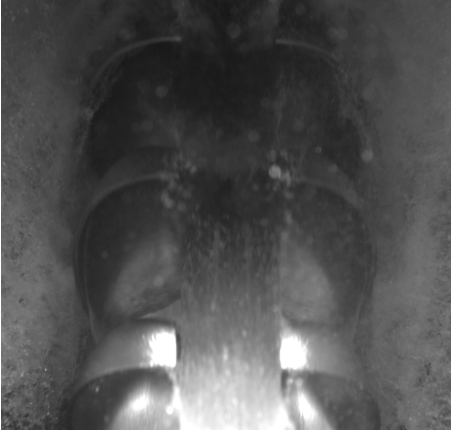
Figure E.47: 70m head, Nozzle opening=14mm, n_{11} = 41
