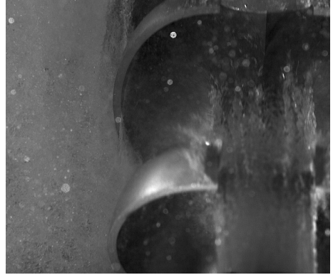
Figure E.12: 70m head, Nozzle open- ing=24mm, n_{11} = 41
