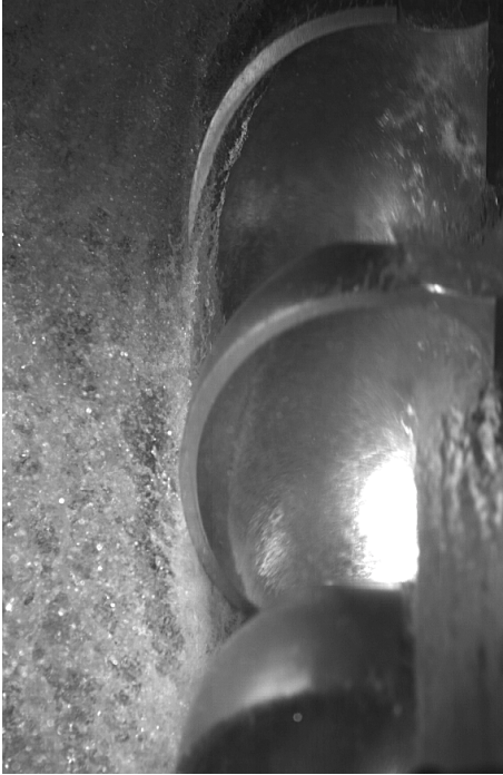
Figure E.1: 70m head, Nozzle opening=14mm, n_{11} = 41
