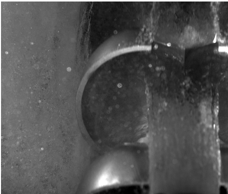
Figure E.13: 70m head, Nozzle open- ing=24mm, n_{11} = 41
