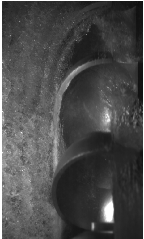
Figure E.6: 70m head, Nozzle open- ing=24mm, n_{11} = 41
