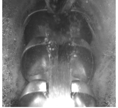
Figure E.44: 70m head, Nozzle open- ing=8mm, n_{11} = 41
