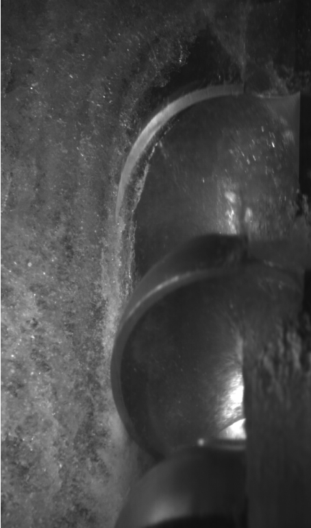
Figure E.7: 70m head, Nozzle opening=24mm, n_{11} = 41
