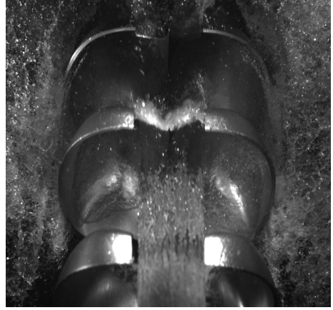
Figure E.32: 25m head, Nozzle open- ing=12mm, n_{11} = 44
