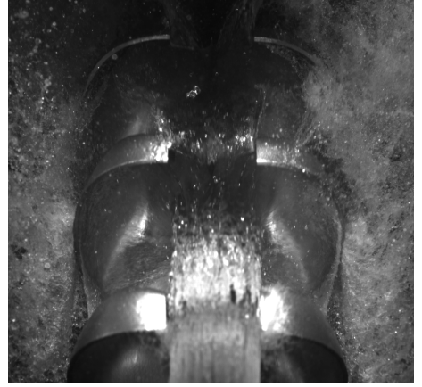
Figure E.20: 25m head, Nozzle open- ing=16mm, n_{11} = 38,5
