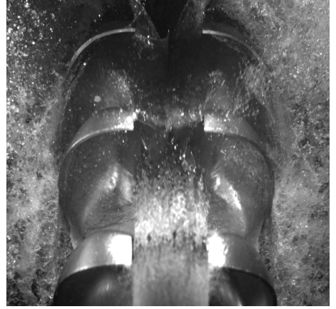
Figure E.28: 25m head, Nozzle open- ing=18mm, n_{11} = 41
