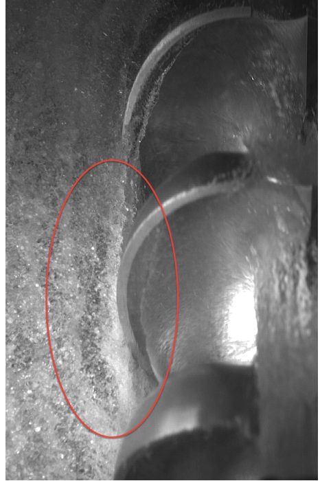
Figure E.2: 70m head, Nozzle opening=18mm, n_{11} = 41
