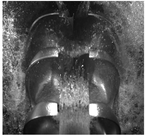
Figure E.26: 25m head, Nozzle open- ing=14mm, n_{11} = 41
