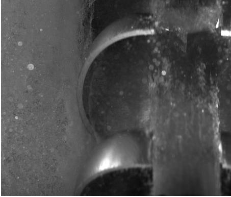
Figure E.11: 70m head, Nozzle open- ing=22mm, n_{11} = 41
