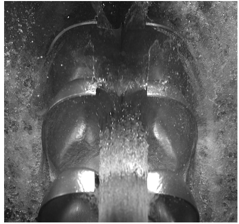
Figure E.18: 25m head, Nozzle open- ing=12mm, n_{11} = 38,5
