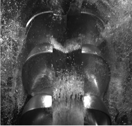
Figure E.35: 25m head, Nozzle opening=18mm, n_{11} = 44
