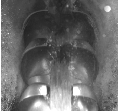
Figure E.43: 70m head, Nozzle open- ing=6mm, n_{11} = 41
