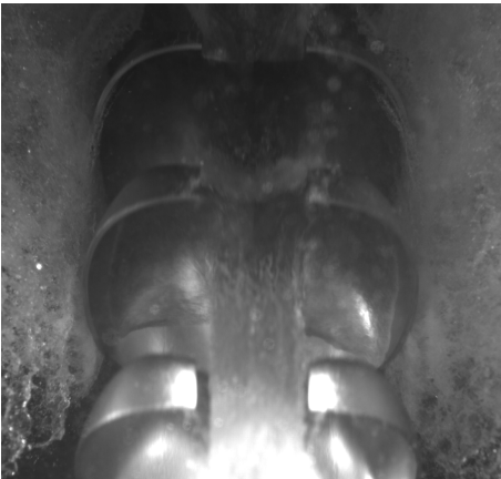
Figure E.37: 70m head, Nozzle opening=8mm, n_{11} = 44
