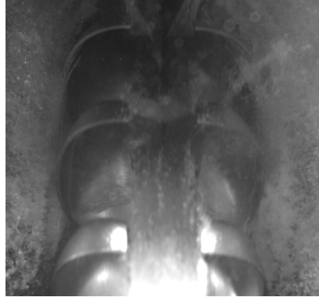
Figure E.40: 70m head, Nozzle opening=14mm, n_{11} = 44
