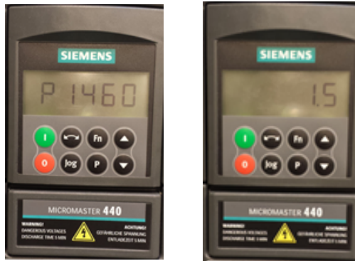
Figure 70: Micromaster code and setting for speed control gain K_p
