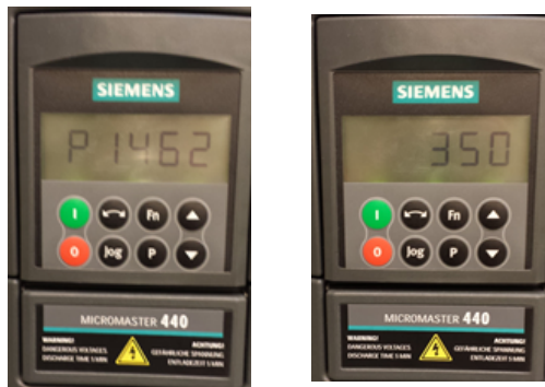
Figure 71: Micromaster code and setting for speed control integrator time T_i
