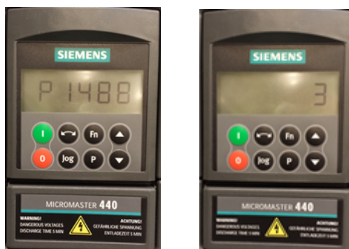
Figure 72: Micromaster code and setting for frequency droop control
