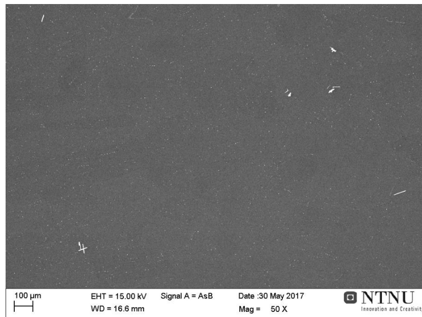
Figure 4.13: The clusters of iron-containing particles are dispersed evenly throughout the material, but the Zr-containing platelets are not.
