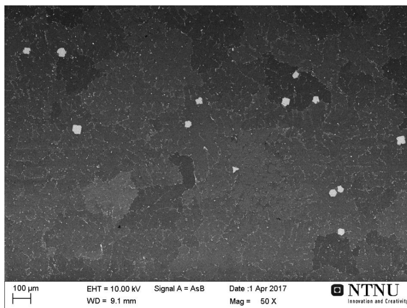
Figure 4.33: Overview image from the AA3003-Mo-Cd sample heated to 550 °C showing larger, Mo-containing particles and finely dispersed Fe- and Mn-containing particles at the grain boundaries.
