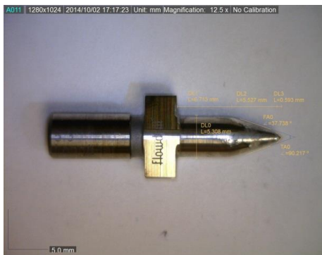
Figure 2 Flowdrill drill bit (5.3 mm diameter)
