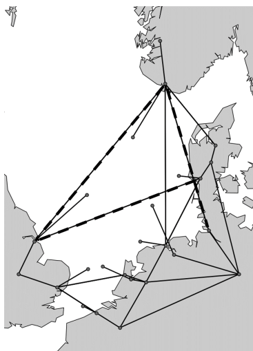
Figure 3: Illustration of the North Sea 2030 case study including all transmission lines that are scheduled to be in operation by year 2030. Candidate branches are shown as dashed lines.
