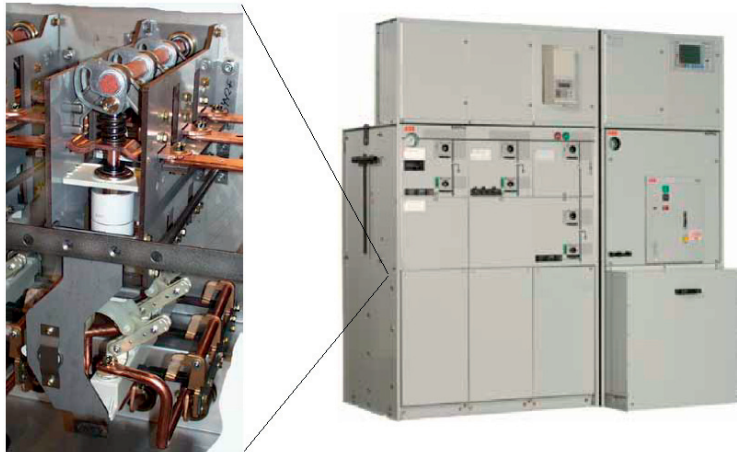
Figure 3.2: Example of \text{SF}_6 filled metal enclosed MV switchgear assembly. Here the LBS is the vacuum type, but \text{SF}_6 -puffer breakers are also common in this application. (Courtesy of ABB, www.abb.com ).
