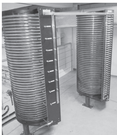
Fig. 5. Load reactor (in the 390 mH setting). The left coil is for coarse tuning and the right coil for fine tuning.
