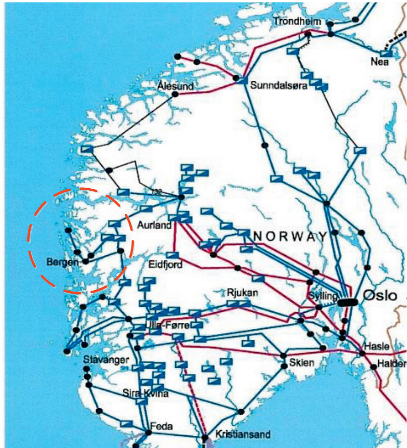
Figure 5.2: Western Norway. The peak load in the subsystem (defined by the red circle) is about 2.5 GW, and the voltage levels in the subsystem are 132kV and 300kV.
