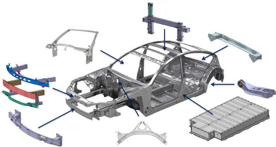
Figure 1.1: Automotive components of extruded aluminum (Benteler Automotive, 2018).
