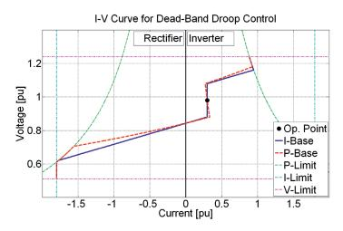
Figure 4.10: *I-V* curve for dead-band droop control
