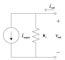
Figure 4.14: Norton equivalent current source of a converter
