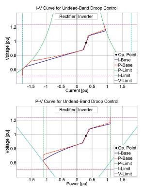
**Fig. 7.** *I–V* curve and *P–V* curve for undead-band droop control.
