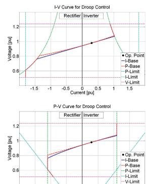
Fig. 2. *I–V* curve and *P–V* curve for droop control.
