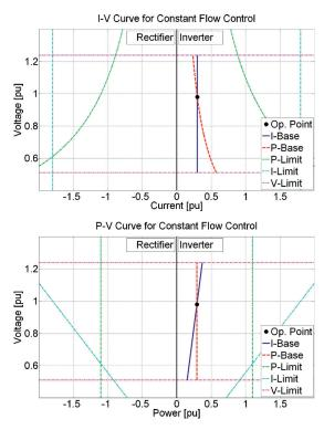
Fig. 3. *I–V* curve and *P–V* curve for constant flow control.
