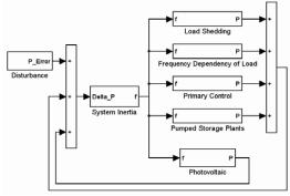
Fig. 5: The UCTE-Frequency Model
