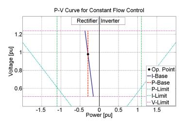
Figure 4.6: *P-V* curve for droop control with infinite droop constant (feeding)
