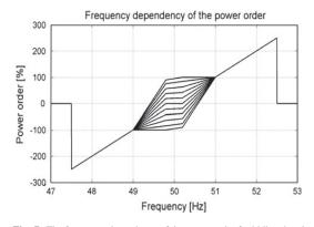
Fig. 7 The frequency dependency of the power order for bidirectional converter systems
