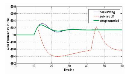
Figure 3.6: Photovoltaic systems influencing the grid frequency
