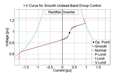
Figure 4.17: I-V curve for smooth undead-band droop control
