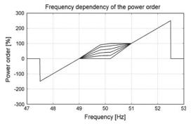
Fig. 3 The frequency dependency of the power order for loads
