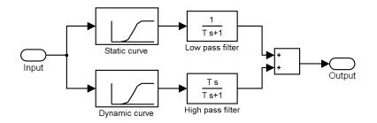
Figure 4.18: Block diagram of improved undead-band droop control
