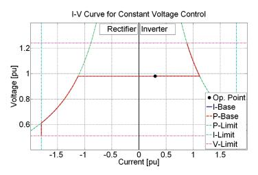
Figure 4.7: *I-V* curve for droop control with zero droop constant
