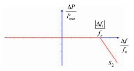
Figure 3.5: Active power frequency response
