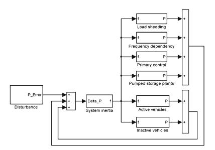
Figure 3.2: Structure of the grid frequency model
