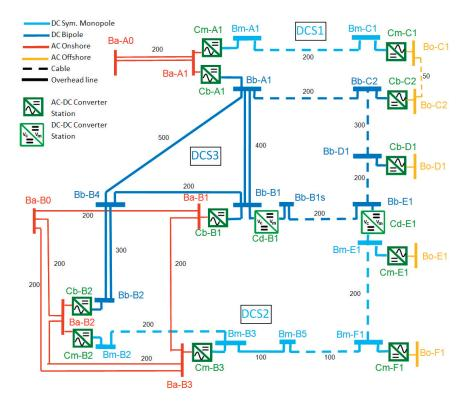
Figure 2.12: The CIGRE B4 DC Grid Test System (detailed)
