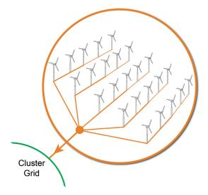
Figure 2.2: Wind power plant collection grid
