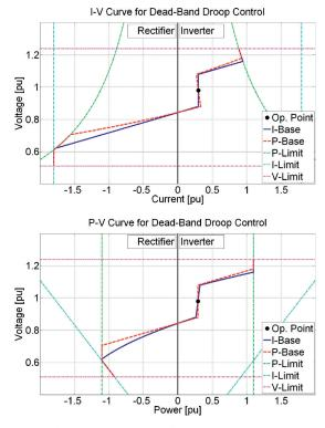
Fig. 6. *I–V* curve and *P–V* curve for dead-band droop control.
