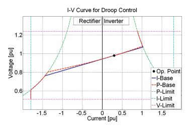
Figure 4.2: *I-V* curve for droop control
