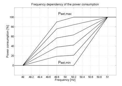
Figure 3.8: Frequency dependent power consumption
