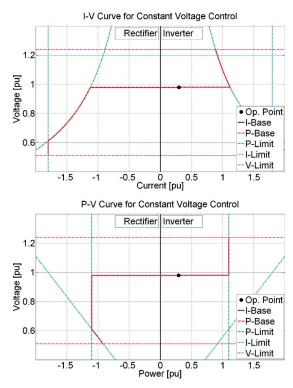
Fig. 4. *I–V* curve and *P–V* curve for constant voltage control.
