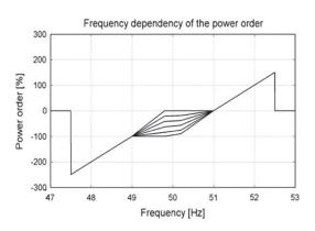
Fig.  $\boldsymbol{6}~$  The frequency dependency of the power order for generation units
