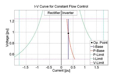
Figure 4.4: I-V curve for droop control with infinite droop constant
