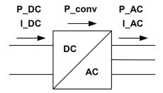
Figure 4.1: Definition of the current & power reference direction
