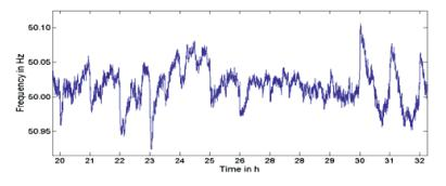
Figure 3.1: Hourly grid frequency spikes
