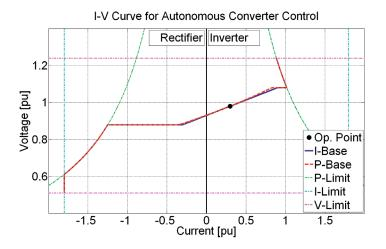
Figure 4.12: I-V curve for autonomous converter control
