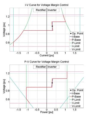
Fig. 5. *I–V* curve and *P–V* curve for voltage margin control.
