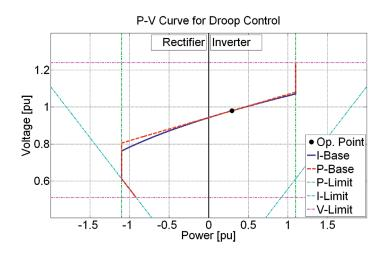
Figure 4.3: P-V curve for droop control
