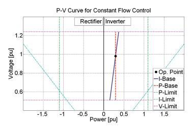
Figure 4.5: P-V curve for droop control with infinite droop constant
