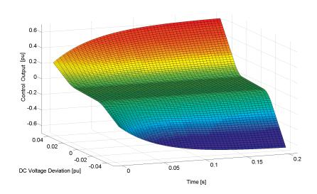
Figure 4.19: Control output as a function of DC voltage deviation and time
