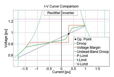
Figure 4.16: Comparison of control methods
