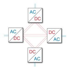
Figure 2.10: Meshed HVDC grid
