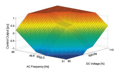
Figure 4.20: Control output as a function of DC voltage and AC frequency
