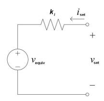
Figure 4.13: Thevenin equivalent voltage source of a converter
