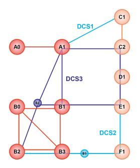
Figure 2.11: The CIGRE B4 DC Grid Test System (schematic)
