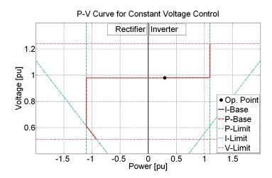
Figure 4.8: P-V curve for droop control with zero droop constant
