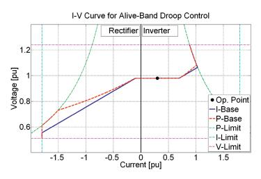
Figure 4.11: I-V curve for alive-band droop control
