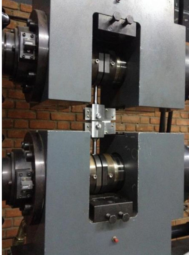
Fig. 6. Configuration of axial fatigue test used for testing CT specimens.
