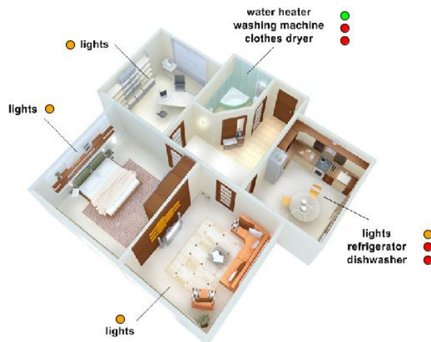
Figure 5.17 State of smart appliances after 3 hours when the water heater is automatically turned on
