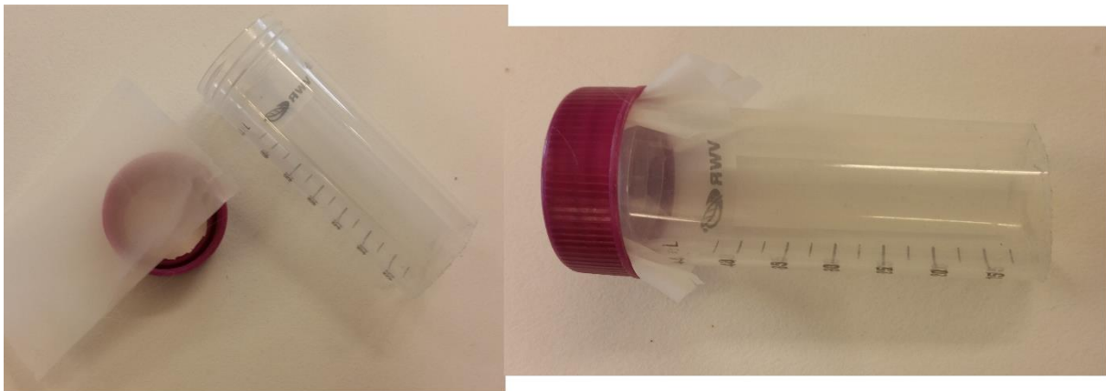
FIGURE 15 SIEVE MADE USING PLANKTON SHEET AND A CUT-OFF PLASTIC VIAL.
