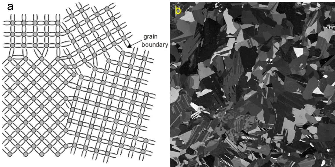
Figure 2.2: a) Multi-Si across the grain boundaries. b) A 10x10cm textured multi-Si wafer. Grains of different orientation appear with different colour. [5]
