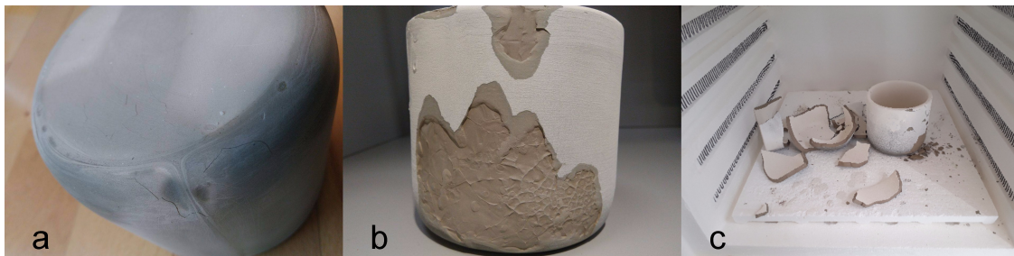
Figure 3.2: Cracks and outer surface flaking of cylindrical crucibles after heat treatment
