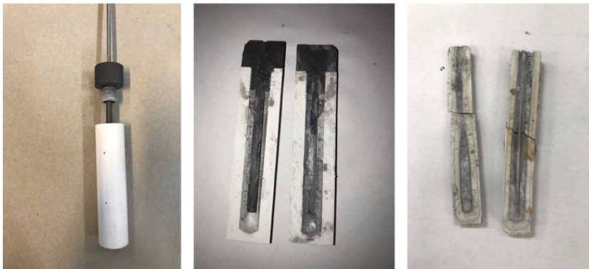
Figure 4.3: Pictures of the reference electrodes. From the left: Graphite reference, spent graphite reference, spent aluminium reference.
