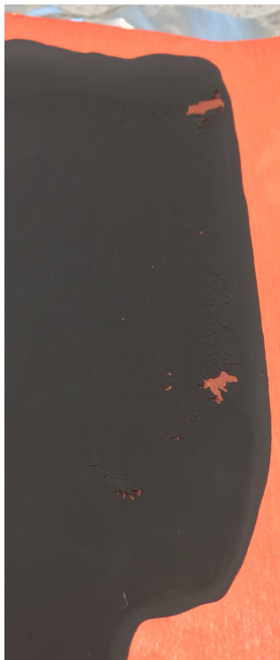
Figure A.4: Brittle part of cast 020616. The dried powder material flaked off.
