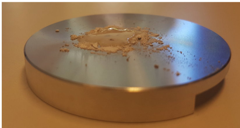
Figure 4.16: Observation image of the hydrophilic properties of the hydrophobisated HSNS sample, HSNShfP(140)12.002.
