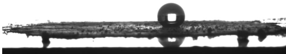
Figure 5.1: Contact angle measurement of the functionalised sample HSNSfP(160)11.551. Notice that the water droplet is not in the center of the solid material.
