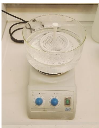
Figure 3.2: Experimental setup for deep etching in heated NaOH.
