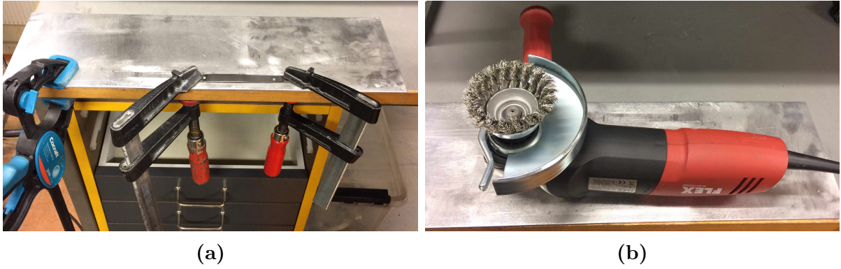
Figure 10: (a) The work-bench for brushing procedure with a sample fastened with clamps. (b) The 0.3mm rotating steel-wire-brush mounted on the hand-held grinder.
