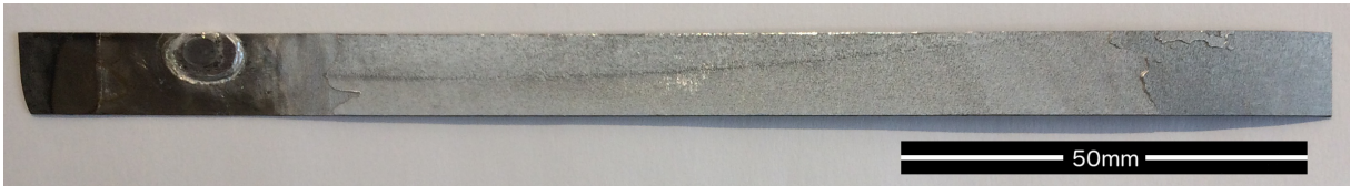
Figure 16: Sample 355_3 after peel-testing. Crack was initiated at left hand side of the sample (where the rivet can be seen) and propagated towards right as the sample was peeled.
