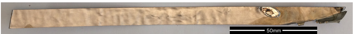
Figure 20: Sample 355Ni_3 after peel-testing. Crack propagated from right hand side (where the rivet can be seen) towards left.
