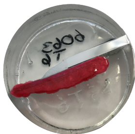
Figure 3.4: Nail polish was used to coat the steel side of the weld to prevent dissolution of steel during anodizing.
