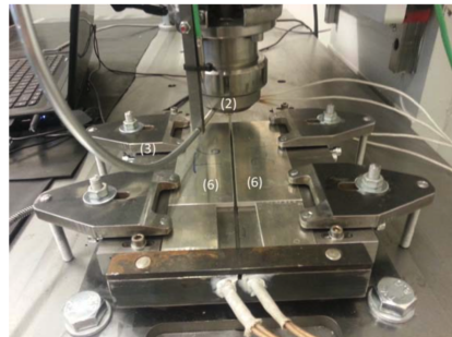
(a) Schematic representation of the HYB process. (b) The setup of the HYB process, where the HYB spindle extruder (2), steel fixture (3) and aluminium test plates (6) are indicated.
