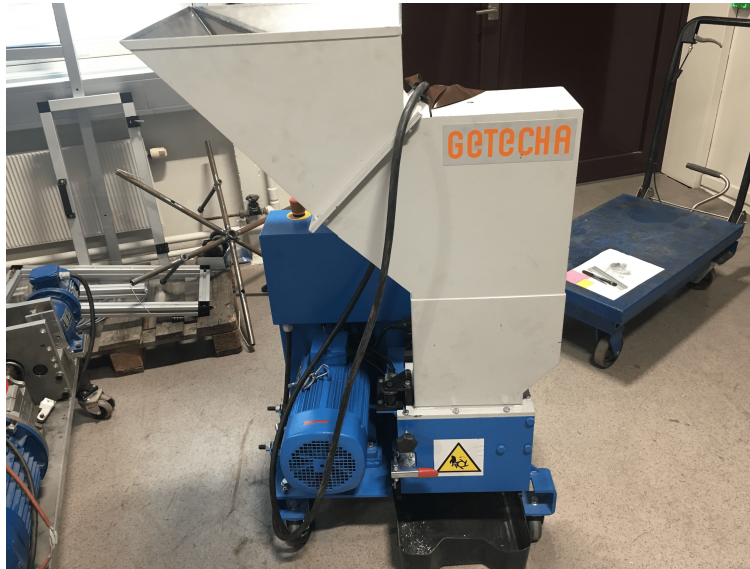
Figure 3.3: Getecha granulator used to granulate aluminium foil.
