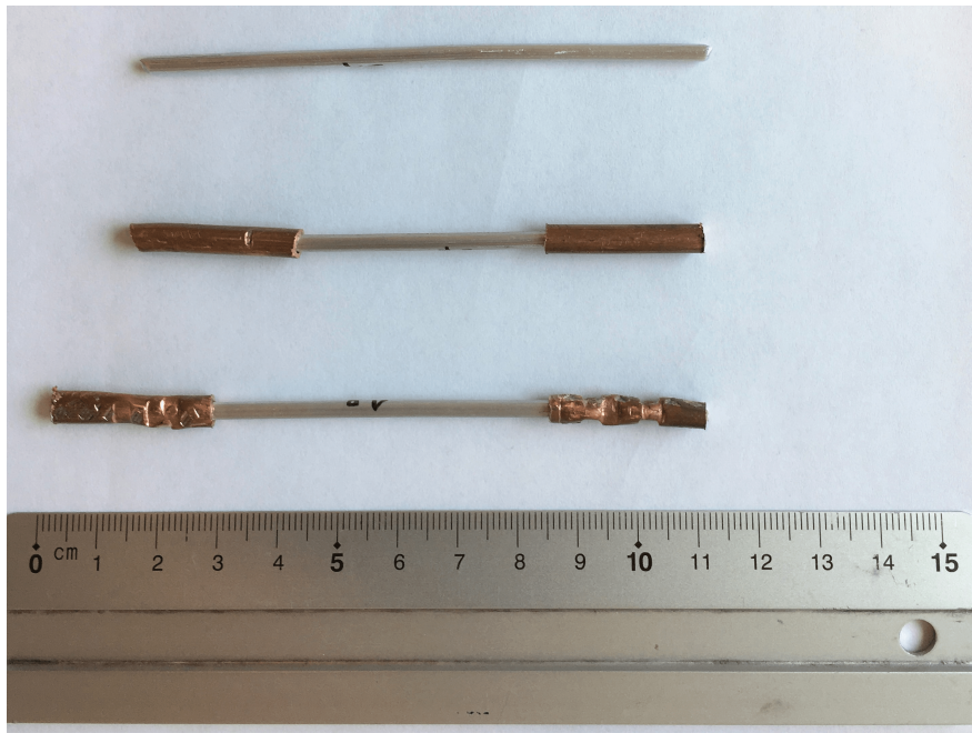
Figure 3.11: Picture of tensile wires for tensile testing of 3mm screw extruded aluminium.
