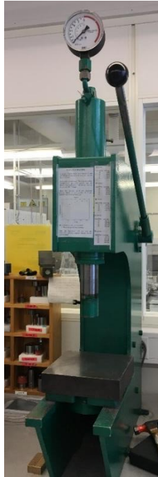
Figure 3.4: Hand press that was used to produce the briquettes
