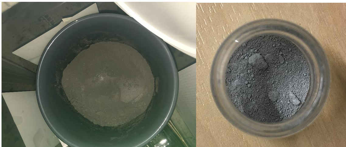
Figure 3.1: Material provided by REC Solar, silicon fines on left, microsilica on right
