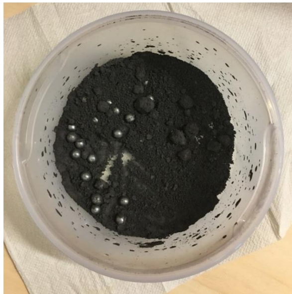
Figure 3.3: Mixing the combination of water and silicon fines with the use of steel balls
