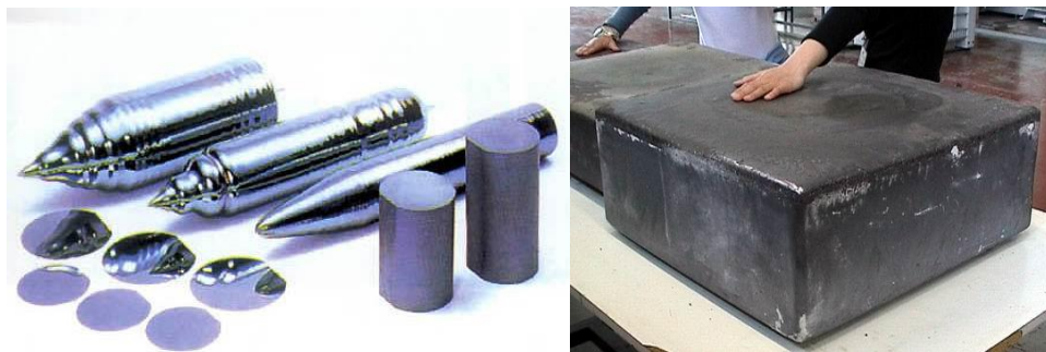
Figure 2.6: Monocrystalline ingot on the left and multicrystalline ingot on the right
