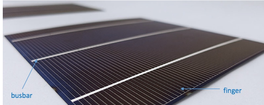
Figure 2.3: Polycrystalline silicon solar cell: busbars and fingers (17) .
