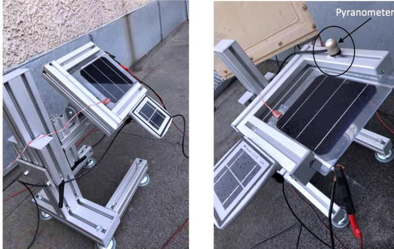
Figure 3.3: The images show the set-up outside, along with how the surroundings looked like. The left image shows 45^\circ tilt angle on the bifacial solar cell. Whereby the right image shows 0^\circ tilt angle on the cell, along with two Pyranometer (one at the top and one beneath, which can not be seen).
