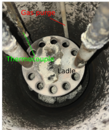
Figure 4.6: Photograph of the setup seen from above.
