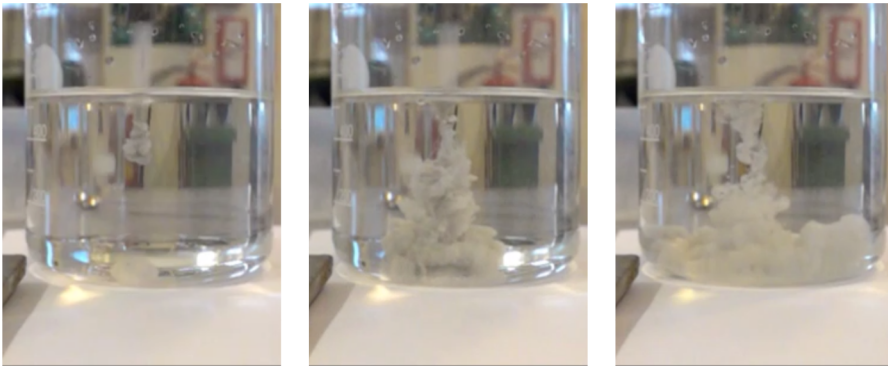
Figure 3.4: Images of alumina fed in a saline solution from a total drop height of 53 cm. Bubbles were observed, but are not visible in the current images.
