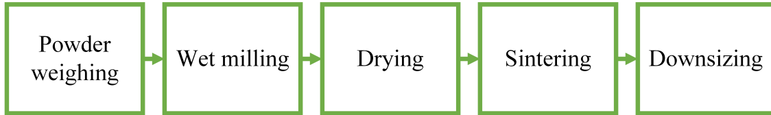
Figure 3.2: Schematic of the processes that are a part of the MAX phase synthesis.
