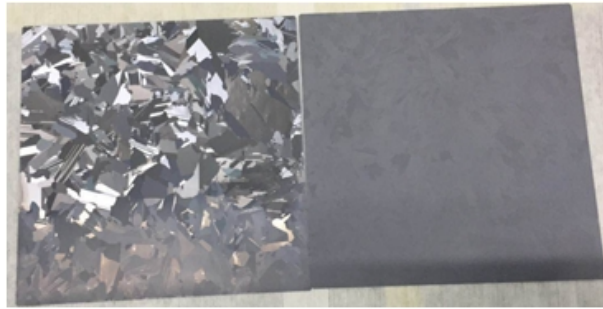
Figure 3.3: The single surface texture process, rear surface to left and front surface to the right.
